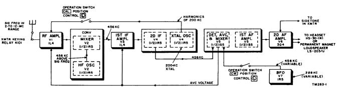
Figure 55. Block diagram of receiver section.
