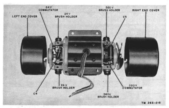
Figure 147. Dynamotor D1, with end covers removed.
