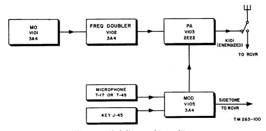
Figure 68. Block diagram of transmitter.
