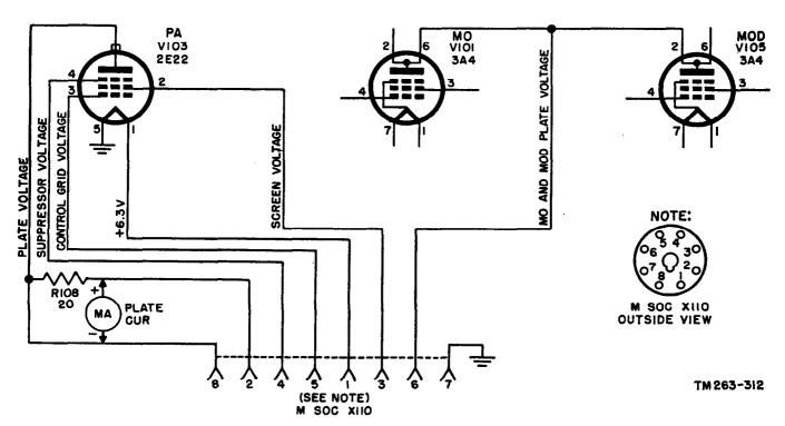
Figure 93. Meter socket X110 connections.
