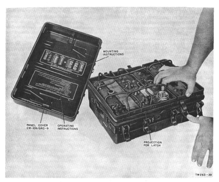
Figure 29. Resetting the latches on receiver-transmitter.
