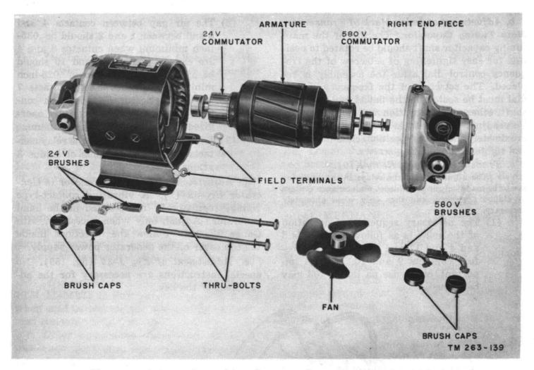
Figure 157. Armature removed from Dynamotor-Power Supply DY-105/GRC-9X.
