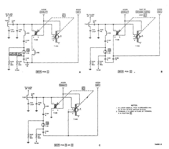
Figure 82. Switch S102, positions 1 through 4.
