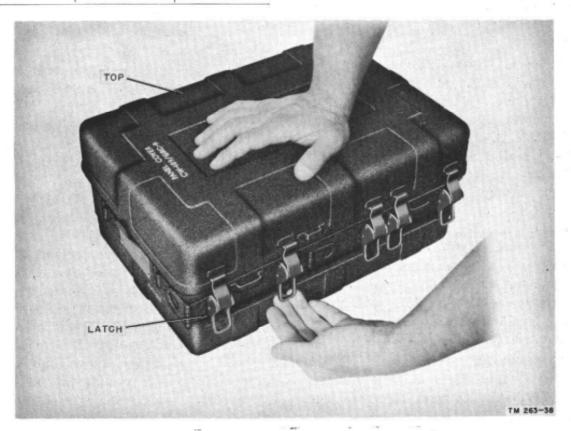
Figure 28. Removing front cover of receiver-transmitter.
