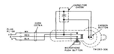
Figure 167. Internal wiring diagram of Microphone T-17.
