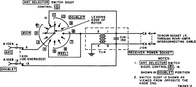
Figure 56. Antenna switching circuit of receiver.
