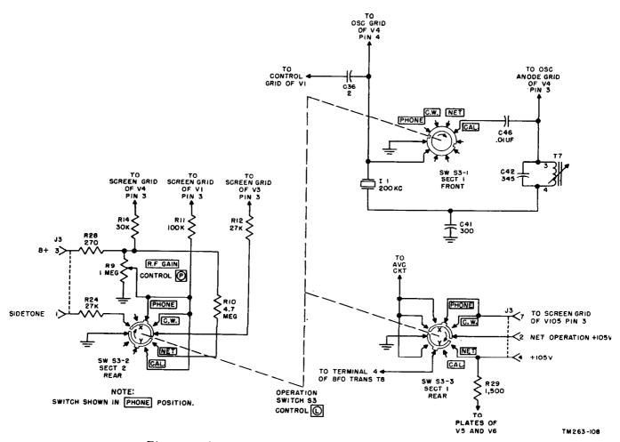
Figure 65. Operation switch S3, simplified schematic diagram.
