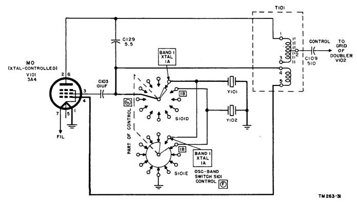
Figure 73. Mo (crystal-controlled), switch sections S101D and S101E.
