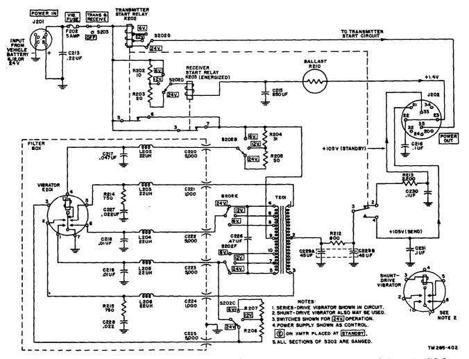
Figure 103. Dynamotor-Power Supply DY-88/GRC-9X vibrator and voltage selector switch S202, simplified schematic diagram.
