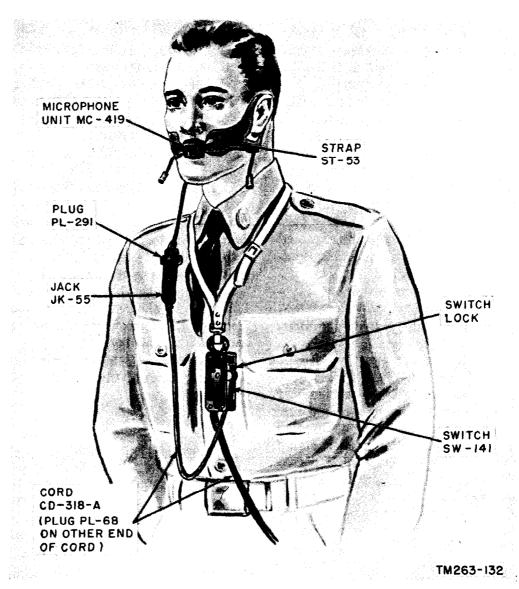
Figure 50. Microphone T-45, in use.
