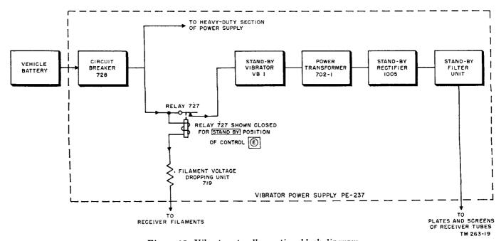
Figure 95. Vibrator standby section, block diagram.
