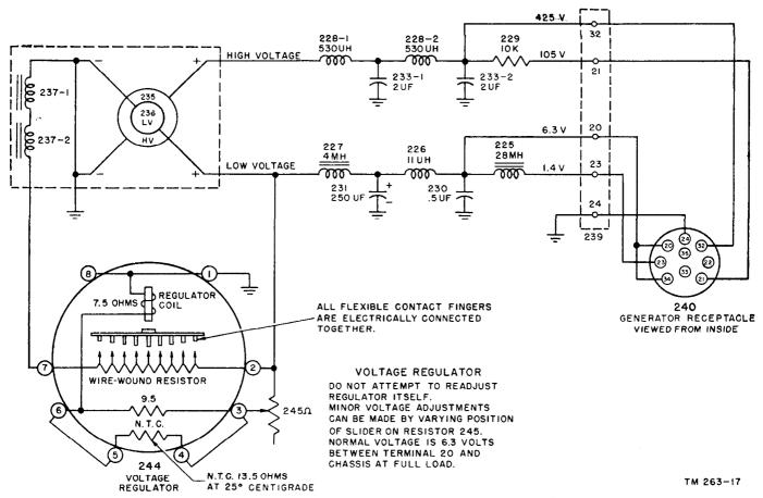
Figure 169. Generator GN-58-A (early models), schematic diagram.
