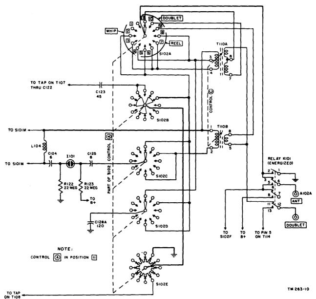
Figure 81. Antenna switching and tuning circuits.
