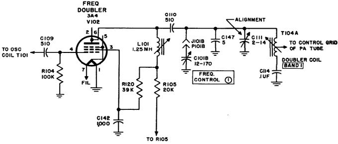
Figure 74. Frequency doubler, simplified schematic diagram.
