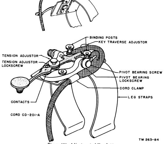
Figure 159. Adjustment of Key J-45.
