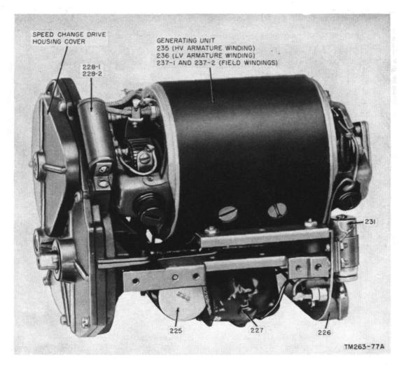
Figure 129. Generator GN-58-A, parts location. (rear).
