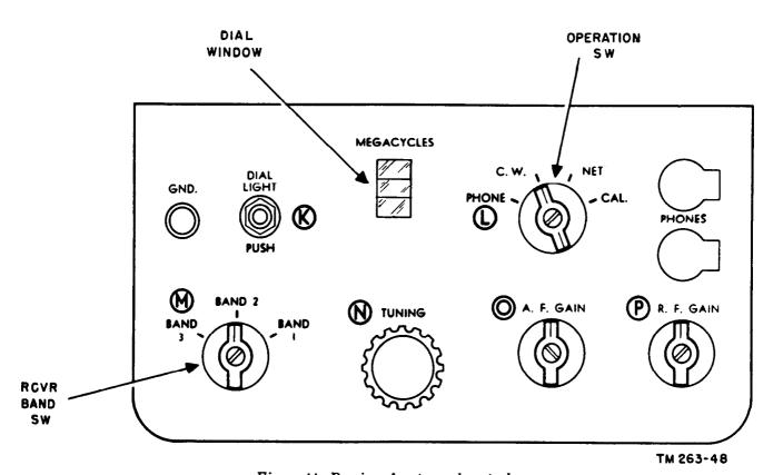
Figure 44. Receiver front panel controls.
