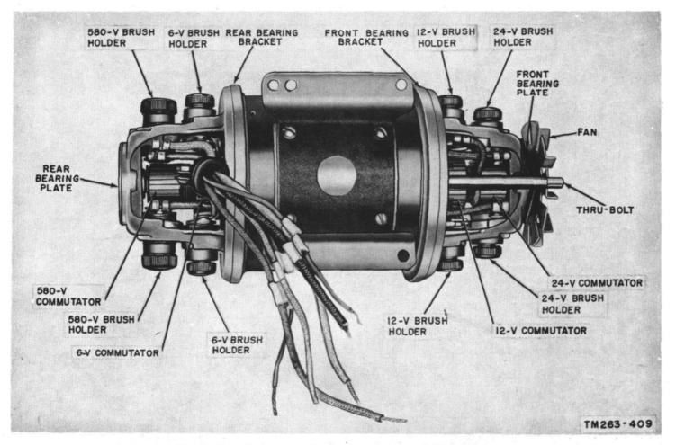
Figure 144. Dynamotor D201, covers removed, bottom view.
