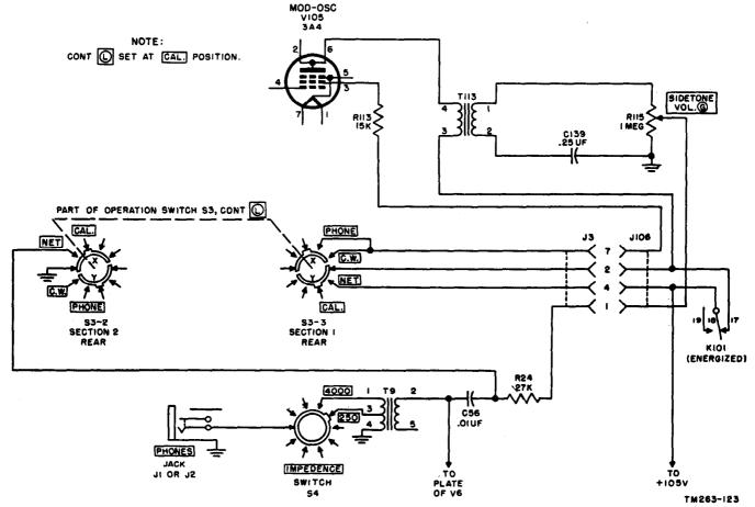
Figure 87. Sidetone switching circuit, simplified schematic diagram.
