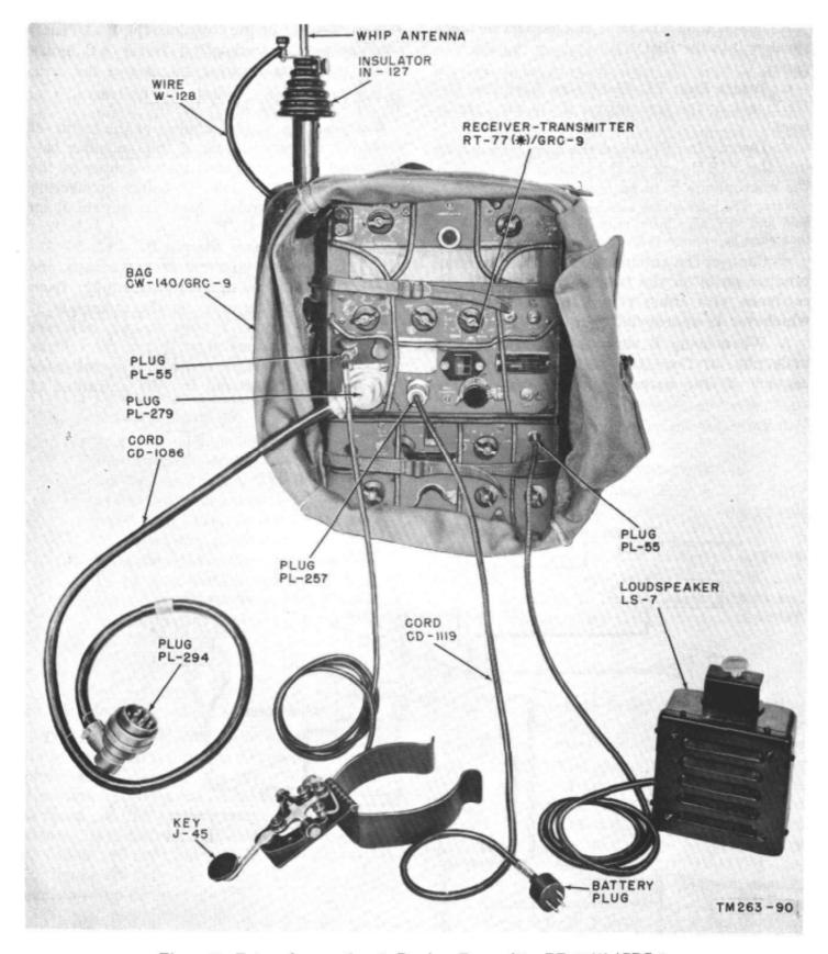
Figure 42. External connections to Receiver-Transmitter RT-77(\*)/GRC-9.
