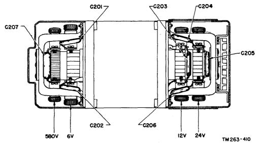
Figure 150. Dynamotor D201, parts location in some models.
