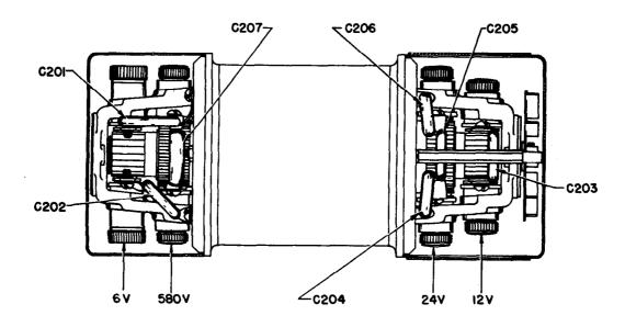
Figure 151. Dynamotor D201, parts location in other models.
