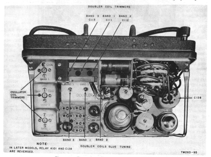
Figure 163. Transmitter alinement points, top of chassis.
