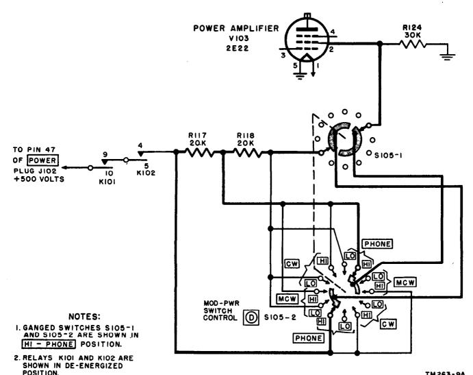
Figure 79. HI power position of control (19), simplified schematic diagram.
