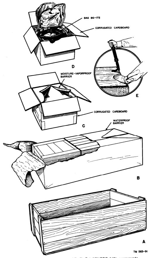
Figure 16. Typical packaging of Radio Set AN/GRC-9 (\*) components.
