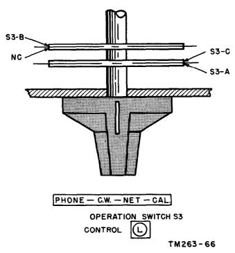
Figure 116. Location of water sections of switch S3.
