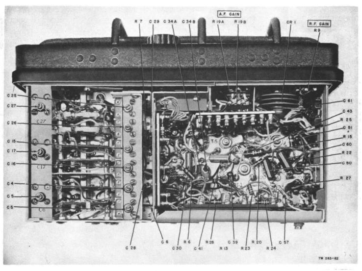
Figure 112. Receiver bottom, parts location.
