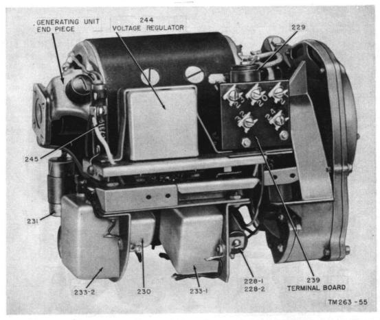
Figure 128. Generator GN-58-A, parts location (front).
