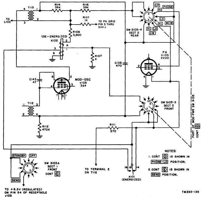
Figure 88. Modulation positions of S105, simplified schematic diagram.
