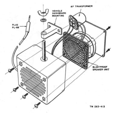
Figure 158. Disassembly of loudspeaker.
