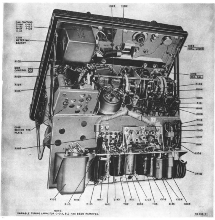
Figure 121. Transmitter parts location (bottom).
