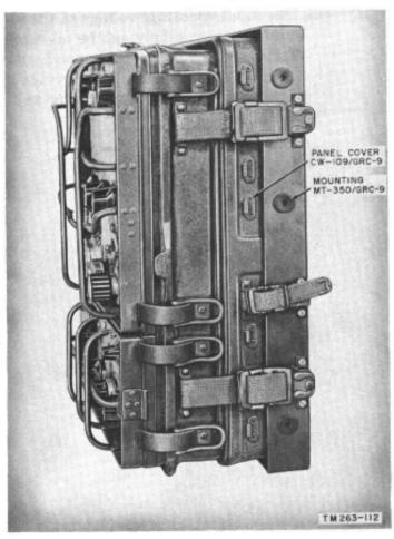
Figure 37. Receiver-transmitter mounted for vehicular use.
