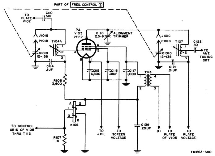
Figure 76. Pa stage, simplified schematic diagram.
