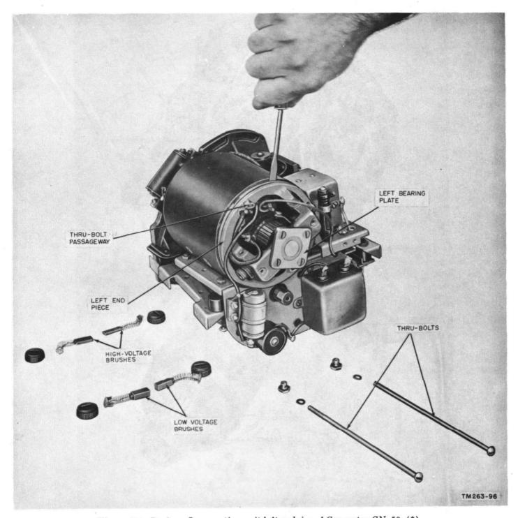
Figure 154. Prying off generating unit left endpice of Generator GN-58-(\*).
