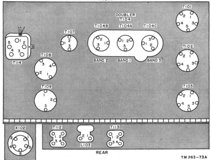
Figure 123. Transformer pin designation on transmitter.
