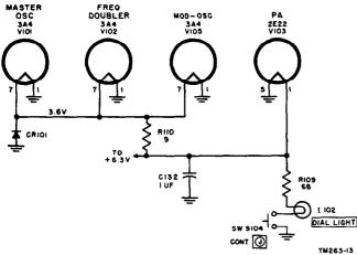
Figure 90. Transmitter filaments, simplified schematic diagram.
