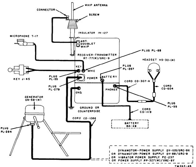
Figure 41. External connections, line drawing.
