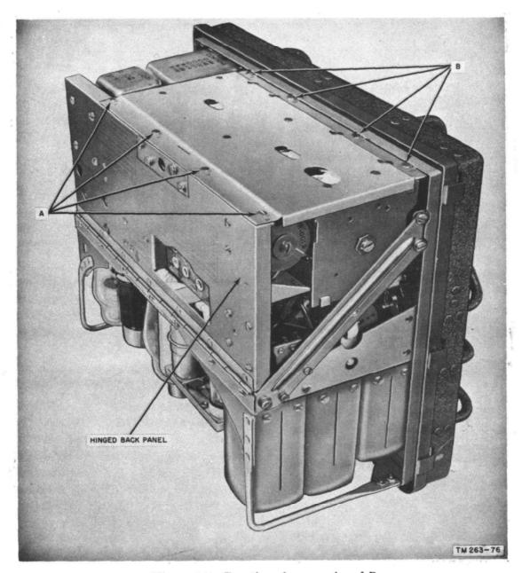
Figure 118. Location of screws A and B.
