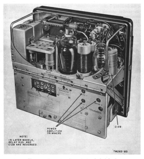
Figure 164. Transmitter alinement points, back of chassis.
