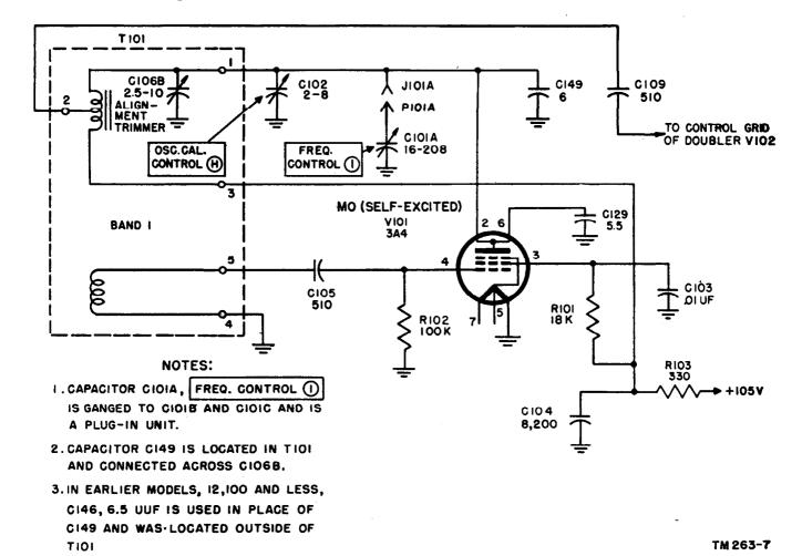
Figure 69. Mo (self-excited), simplified schematic diagram.
