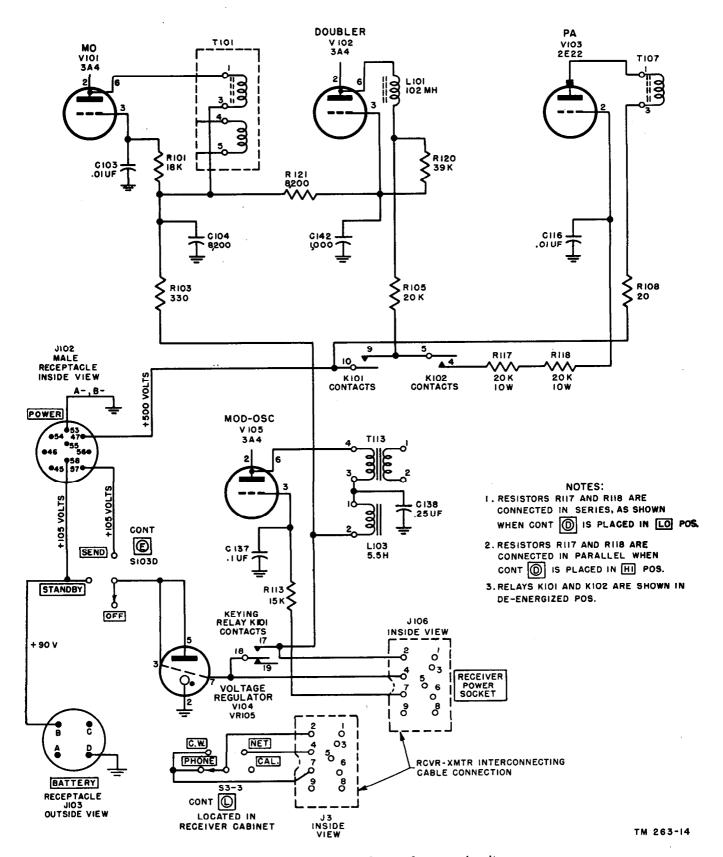
Figure 91. Transmitter plate and screen circuits.
