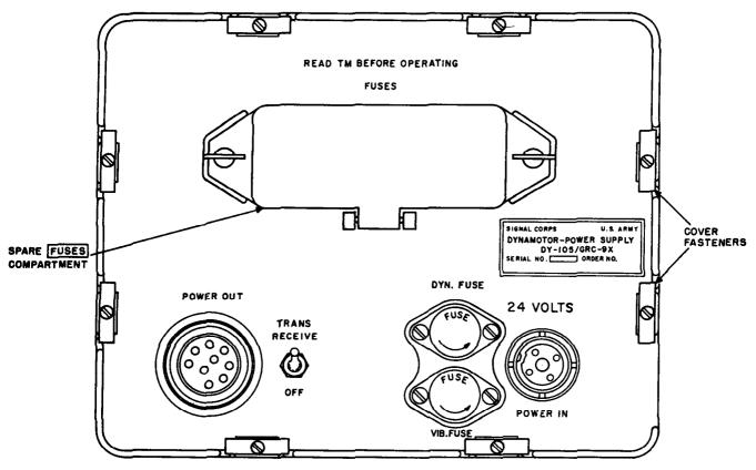
Figure 46. Dynamotor-Power Supply DY-105/GRC-9X, front panel controls.
