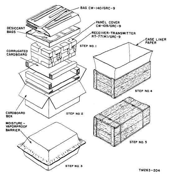
Figure 17. Method of packaging receiver-transmitter section.
