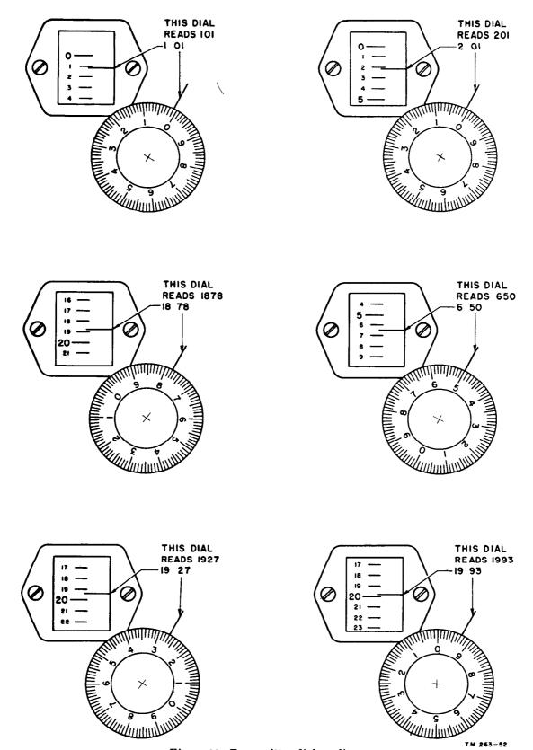
Figure 48. Transmitter dial readings.
