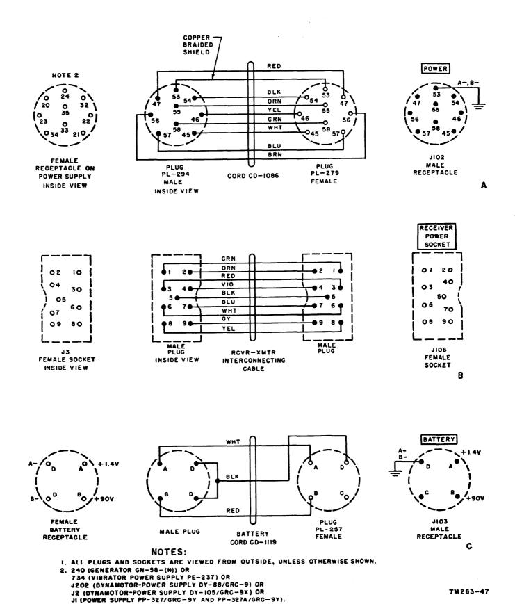
Figure 54. Internal wiring diagrams of cords.
