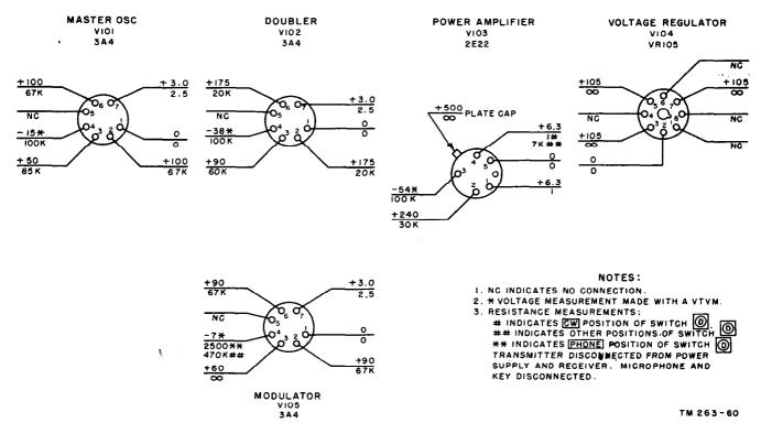
Figure 124. Transmitter tube socket voltage and resistance diagram.
