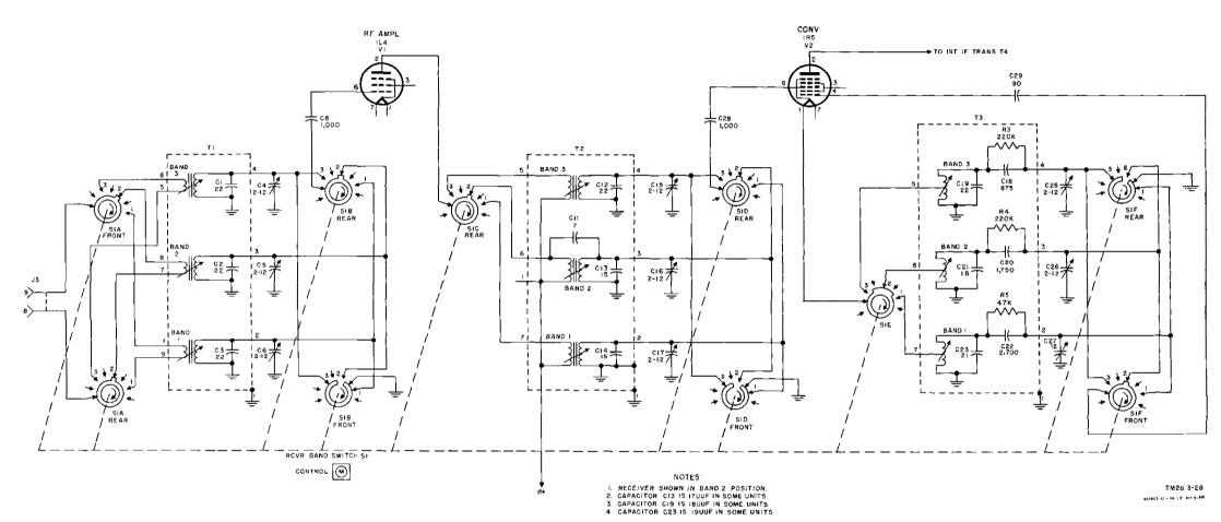
Figure 59. Band changing circuit, simplified schematic diagram
