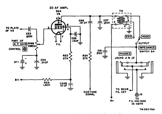
Figure 63. Second audio amplifier, simplified schematic diagram.
