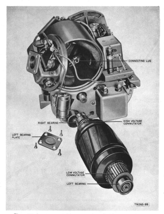
Figure 155. Armature removed from generating unit of Generator GN-58-(\*).
