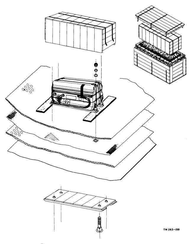
Figure 15. Method of packing typical component for shipping.
