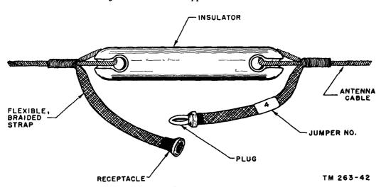
Figure 21. Typical antenna jumper.
