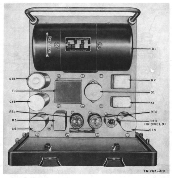
Figure 145. Dynamotor-Power Supply DY-105/GRC-9X, top view of chassis.
