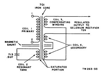
Figure 100. Constant voltage transformer 701.
