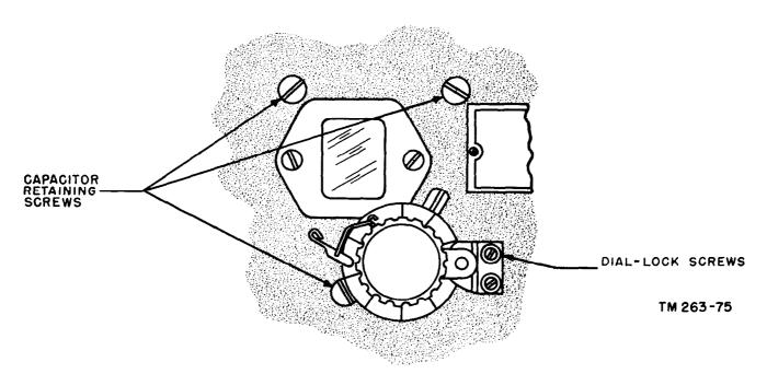
Figure 117. Transmitter capacitor and dial retaining screws.
