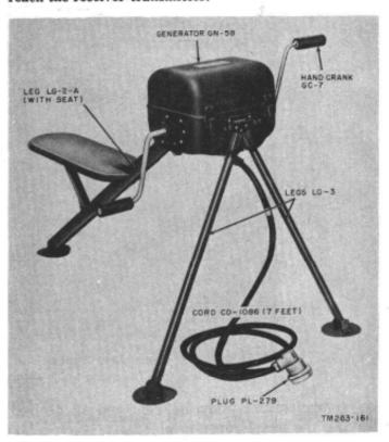
Figure 33. Generator GN-58 set up for operation.
