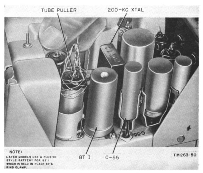
Figure 31. Removing tubes using tube puller.
