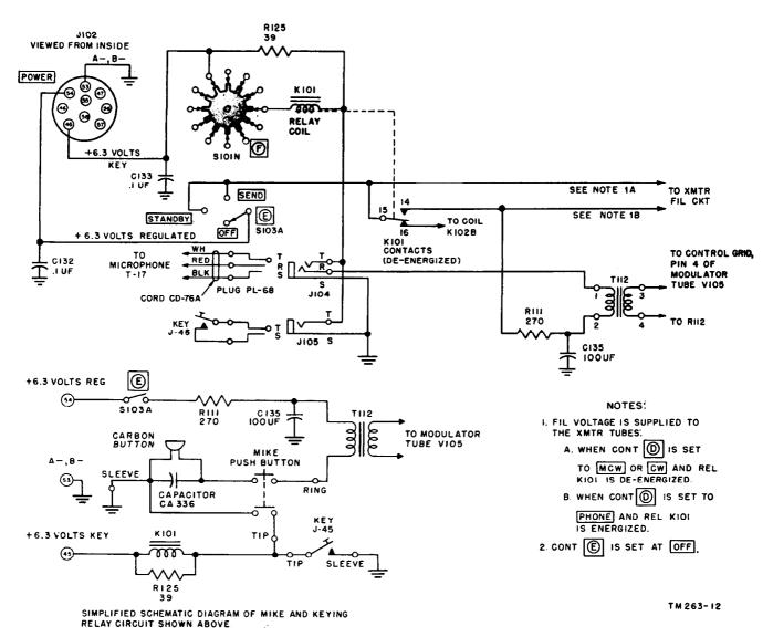
Figure 89. Microphone and key connections.
