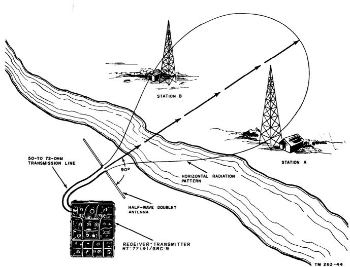
Figure 27. Orientation of half-wave doublet antenna for maximum range.
