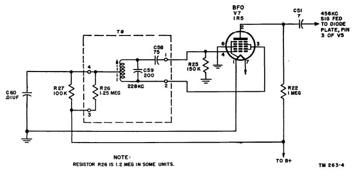
Figure 64. Beat-frequency oscillator, simplified schematic diagram.
