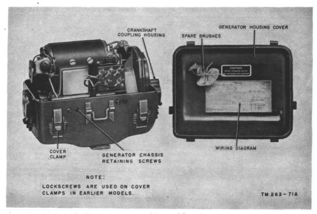
Figure 126. Generator GN-58-(\*), top cover removed.
