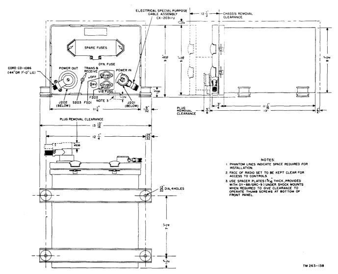
Figure 40. Dynamotor-Power Supply DY-88/GRC-9, outline dimensions and clearances.
