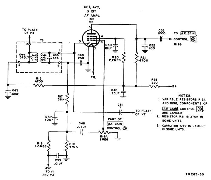
Figure 62. Detector, avc, and first audio amplifier, simplified schematic diagram.
