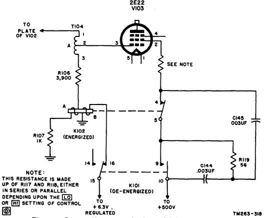
Figure 80. Screen grid protective circuit, simplified schematic diagram.
