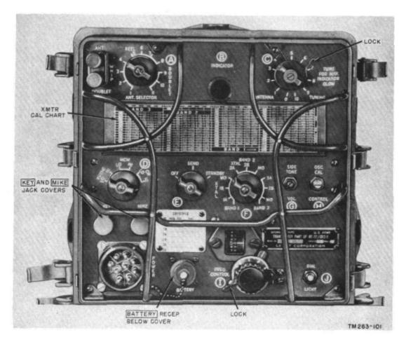
Figure 9. Transmitter section of radio set.
