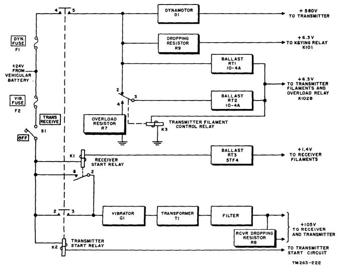
Figure 105. Dynamotor-Power Supply DY-105/GRC-9X, block diagram.
