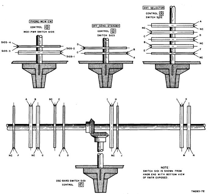
Figure 125. Transmitter wafer switch sections.
