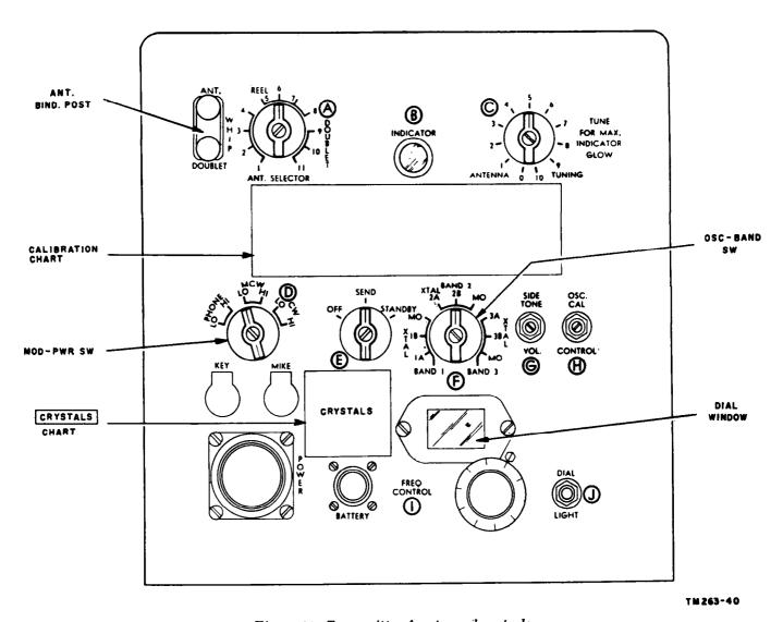
Figure 43. Transmitter front panel controls.
