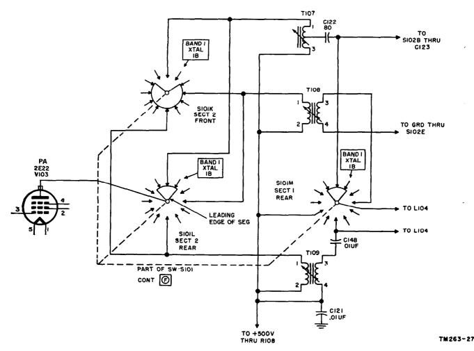
Figure 77. Pa switch sections S101K, S101L, and S101M, simplified schematic diagram.
