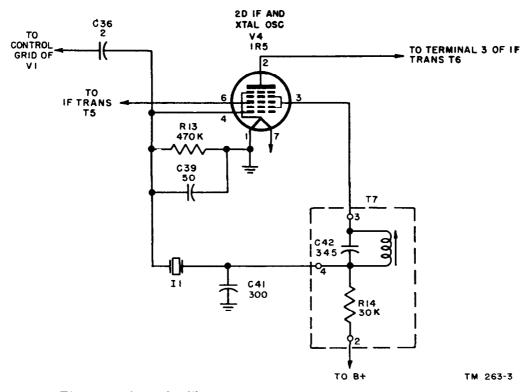
Figure 61. Crystal calibrator ocsillator, simplified schematic diagram.
