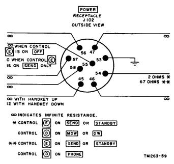
Figure 109. Transmitter POWER socket resistances to ground.
