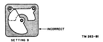
Figure 162. Determination of correct settings of oscillator trimmer capacitor C25, C26, and C27.
