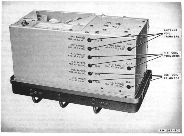
Figure 161. Receiver bottom, alinement points.
