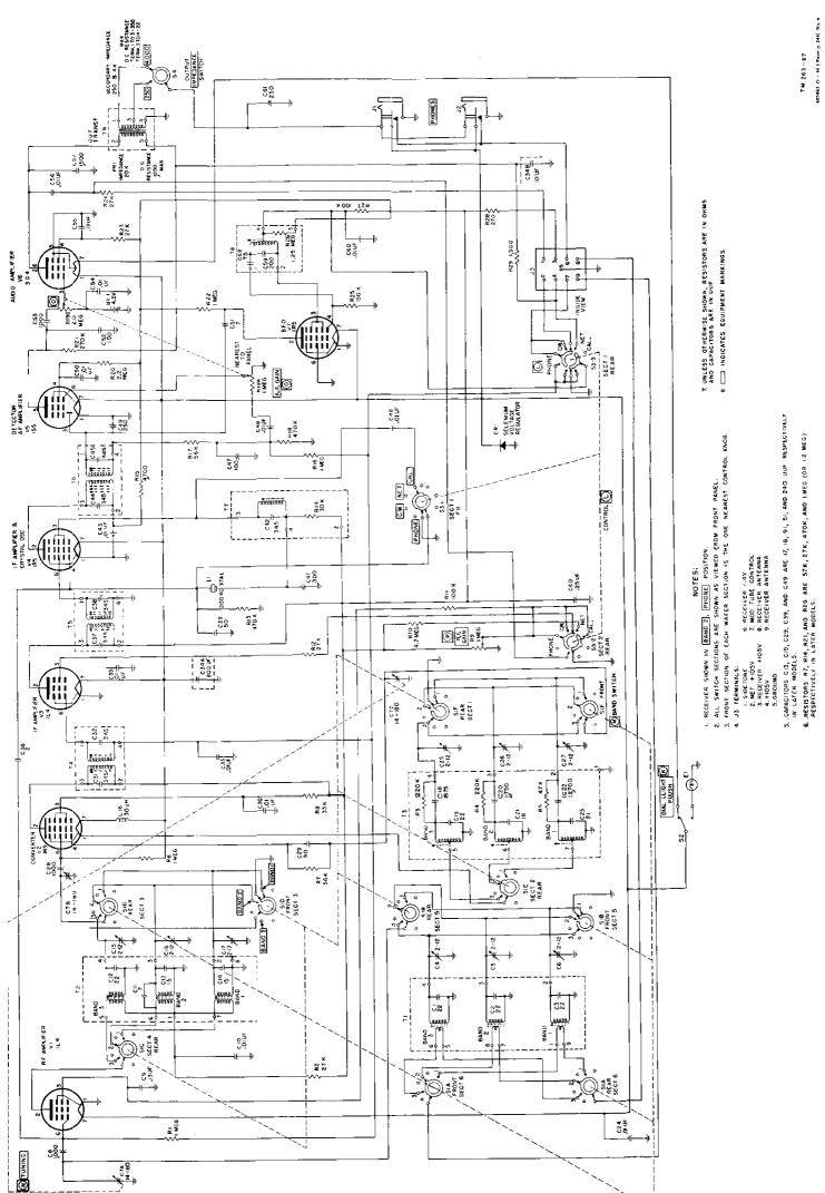
Figure 175. Receiver section, schematic diagran
