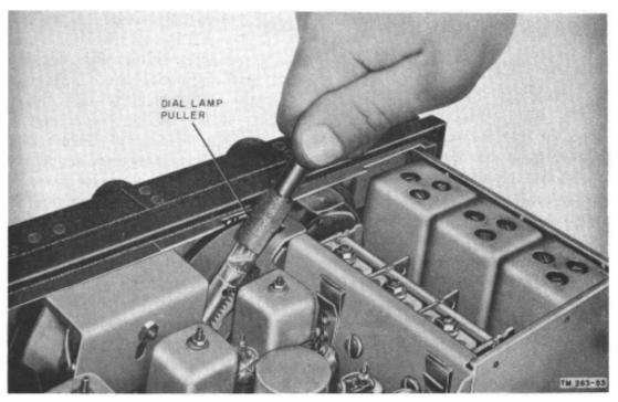
Figure 32. Removing dial lamp using pilot lamp puller.
