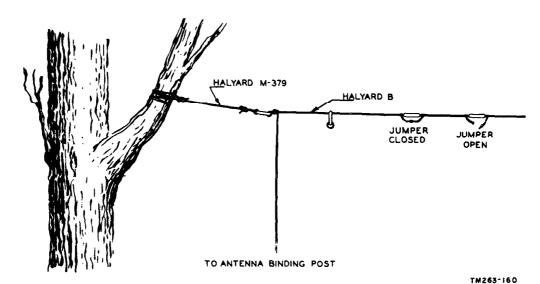
Figure 20. Antenna supports and connections.
