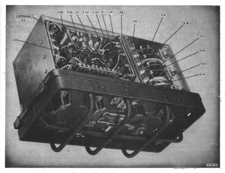
Figure 114. Receiver bottom, parts location.
