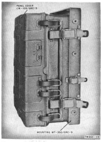
Figure 38. Receiver-transmitter mounted for vehicular transportation or storage.
