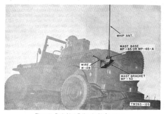
Figure 39. Typical installation of vehicular antenna.
