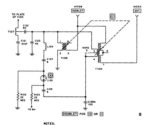
Figure 84. Switch S102, positions 9 through 11.
