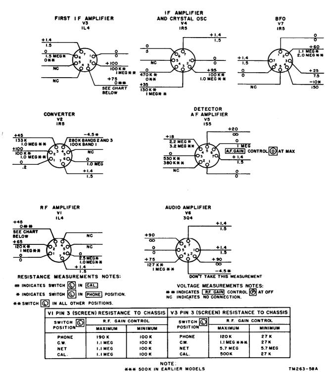
Figure 115. Receiver tube socket, voltage and resistance diagram.
