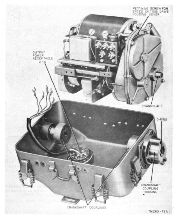
Figure 127. Generator GN-58-A, bottom half of housing removed.
