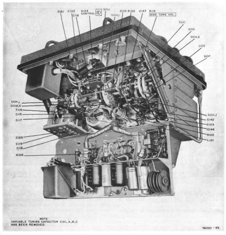
Figure 122. Transmitter parts location (bottom).
