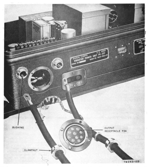
Figure 131. Vibrator Power Supply PE-237, battery cables and power output receptacle 734.
