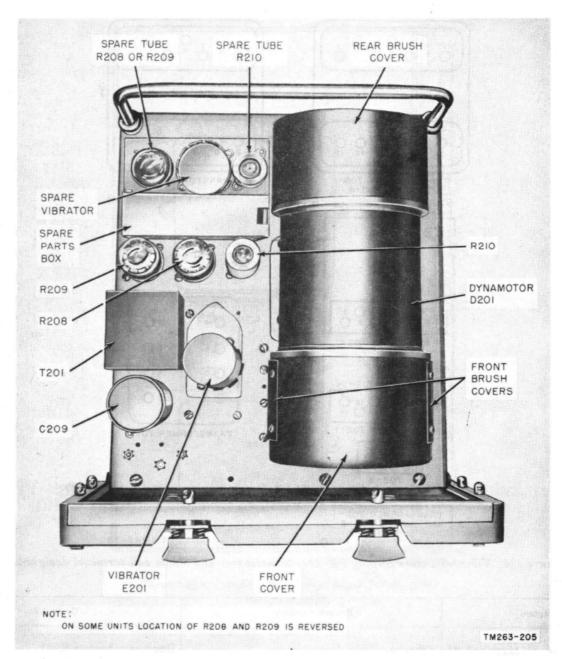
Figure 141. Dynamotor-Power Supply DY-88/GRC-9, top view of chassis.
