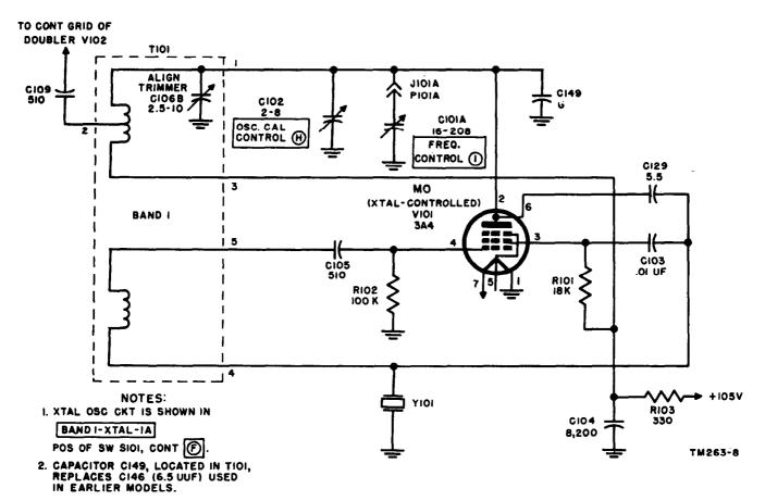
Figure 70. Mo (crystal-controlled), simplified schematic diagram.
