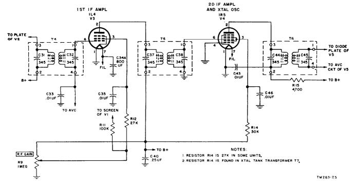
Figure 60. If. amplifiers, simplified schematic diagram.
