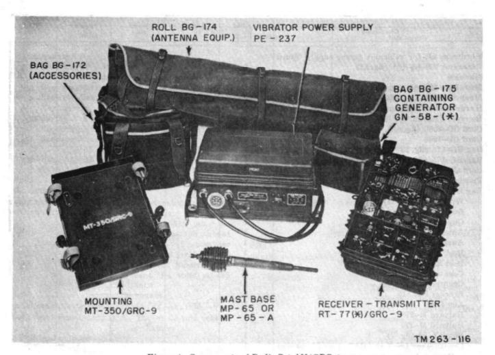
Figure 4. Components of Radio Set AN/GRC-9.
