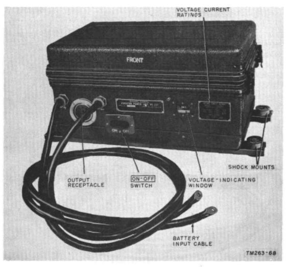
Figure 10. Vibrator Power Supply.
