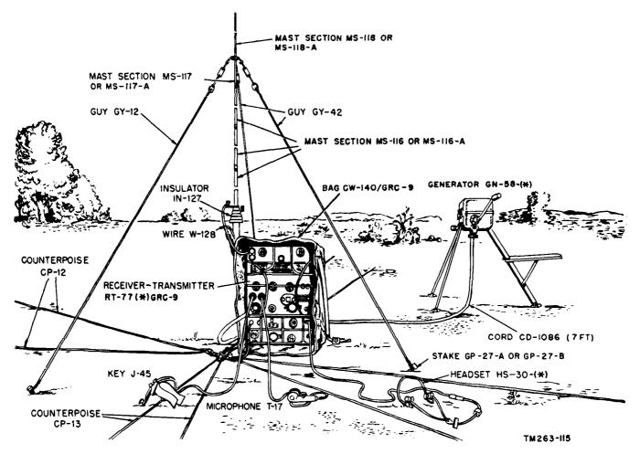
Figure 23. Typical ground installation, whip antenna.
