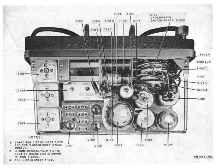
Figure 120. Transmitter parts location (top).
