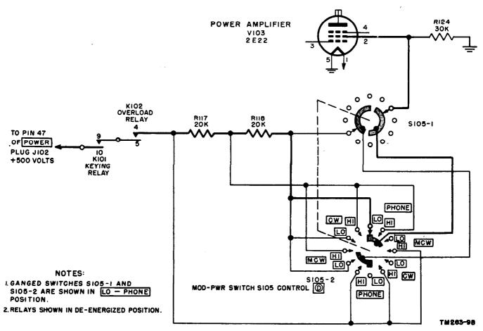
Figure 78. LO power position of control D, simplified schematic diagram.
