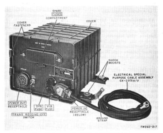
Figure 12. Dynamotor-Power Supply DY-105/GRC-9X.
