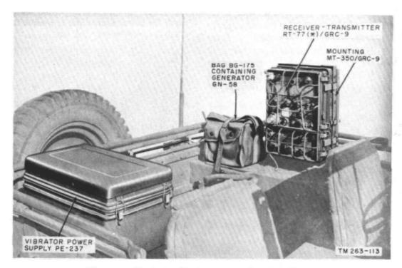
Figure 34. Typical vehicular installation of radio set.
