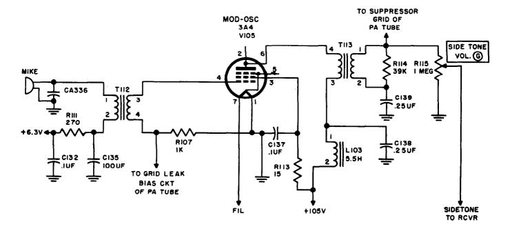
Figure 85. Modulator (voice) stage, simplified schematic diagram.
