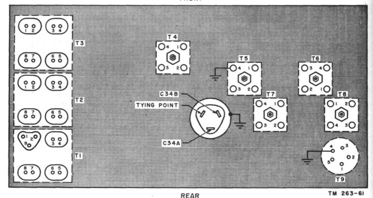
Figure 111. Receiver transformer and electrolytic capacitor terminal designations.
