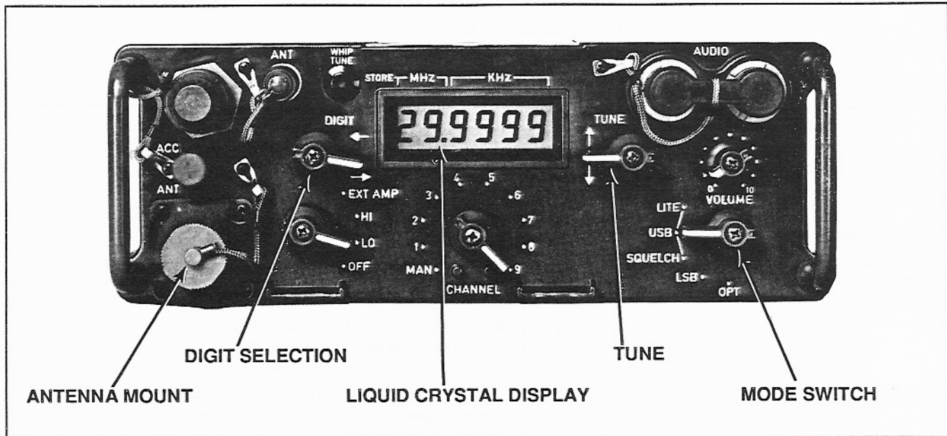
FIGURE 3-1. Transceiver Radio PRC1099, Controls, Indicators, and Connectors.
