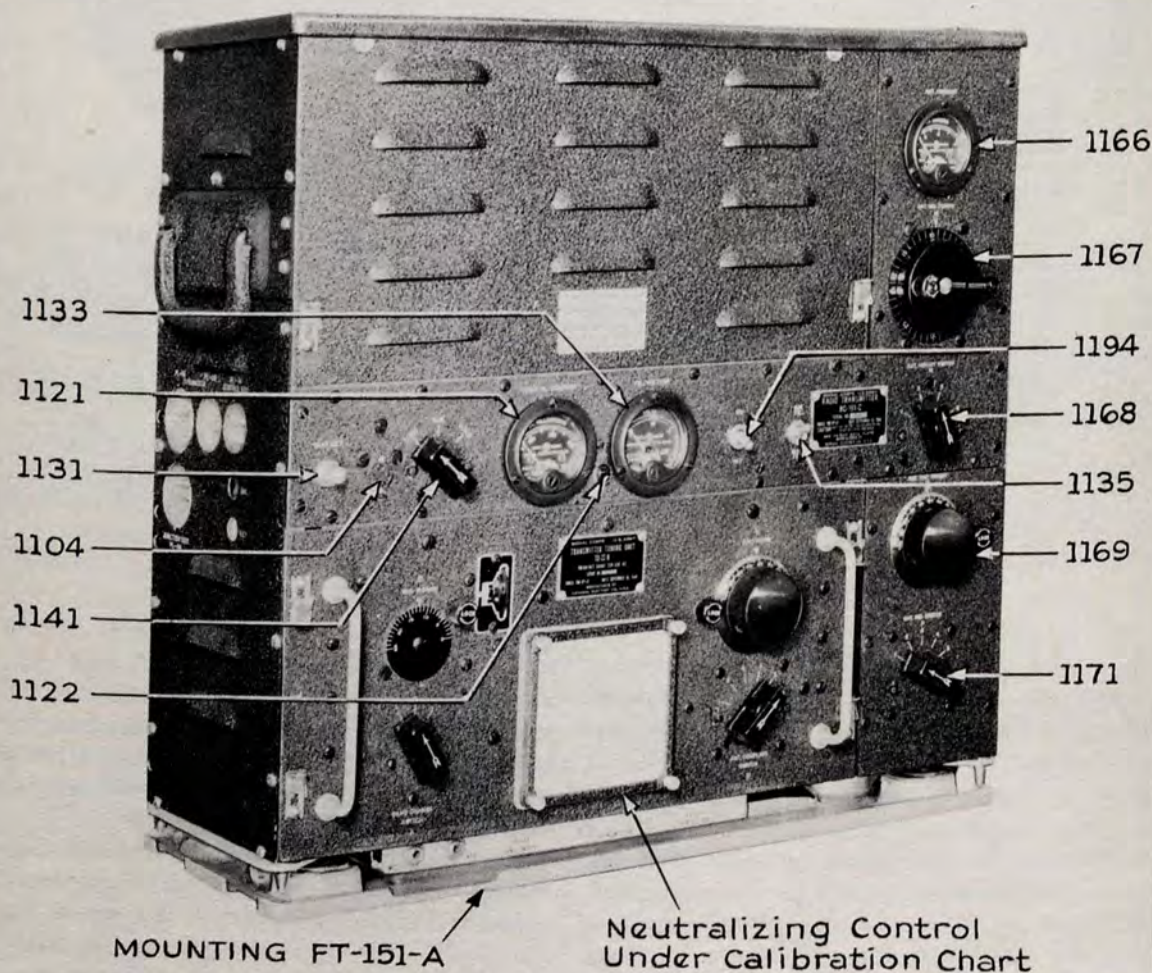
FIG. 6. RADIO TRANSMITTER BC-191-C WITH TRANSMITTER TUNING UNIT TU-22-B IN PLACE
