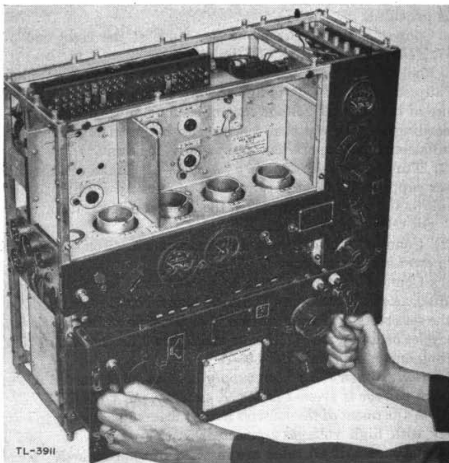
FIGURE 6.—Radio transmitter BC-191-(*)—removing transmitter tuning unit.
