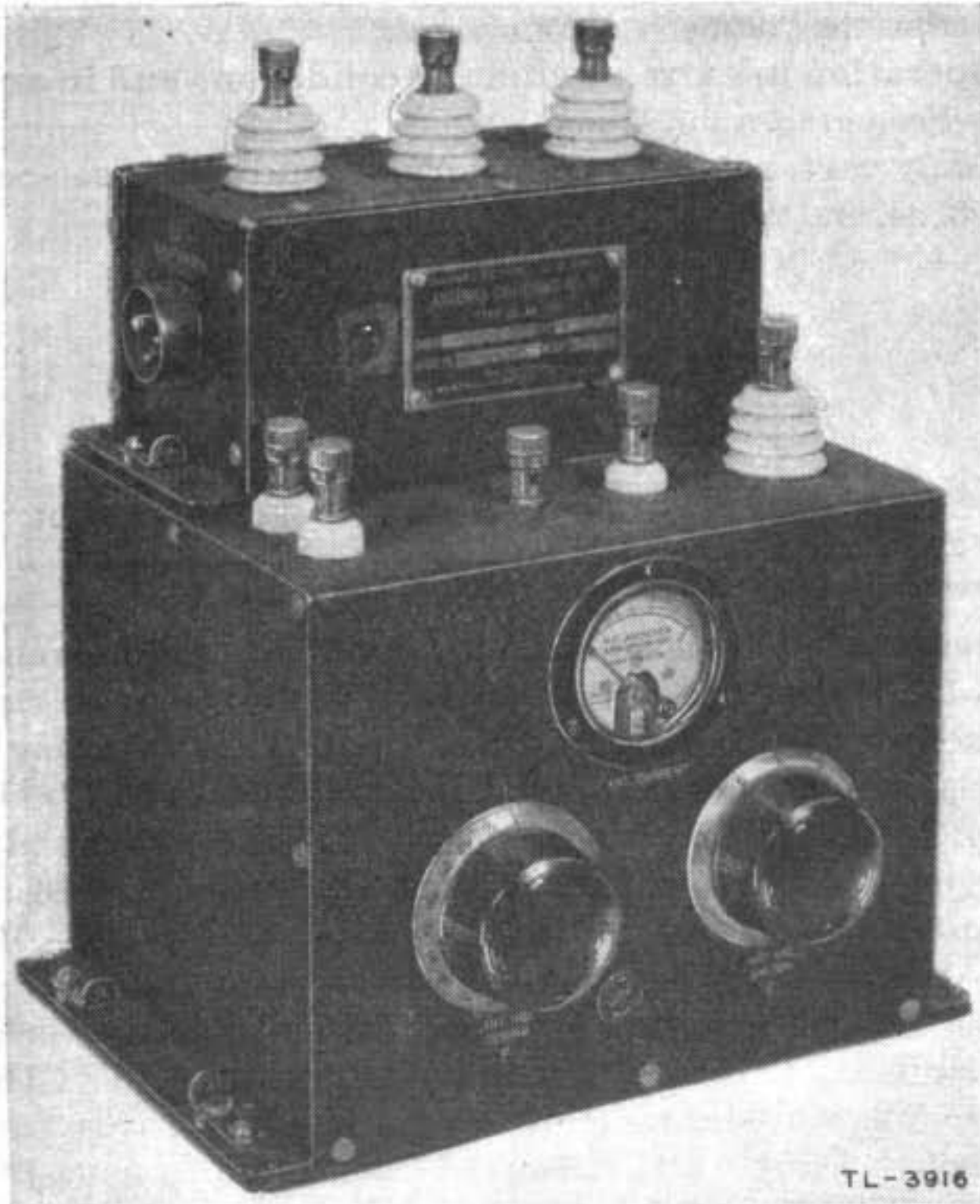
FIGURE 30.—Antenna tuning unit BC-(*)-193 or BC-AA-204 with antenna switching relay BC-(*)-196 mounted on top.
