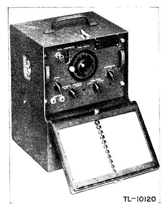
Figure 1. Frequency Meter BC-221-( $\mathfrak{F}$ ), in metal cabinet.
