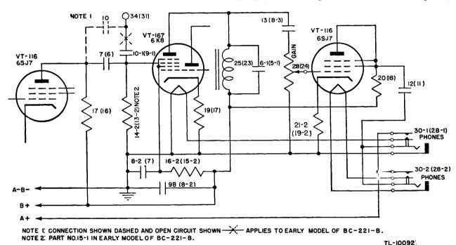
Figure 39. Frequency Meter BC-221-(2), functional diagram, detector and audio-amplifier circuits.
