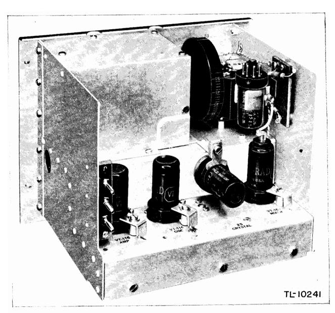
Figure 24. Frequency Meter BC-221-AA, rear view of chassis.
