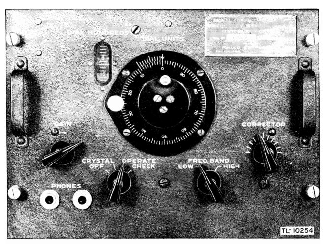
$Figure \ 4. \quad Frequency \ Meters \ BC-221-B, \ BC-221-E, \ BC-221-N, \ BC-221-Q, \ BC-221-AA, \ BC-221-AE, \ and \ BC-221-AG, \ control \ panel \ lay-out.$
