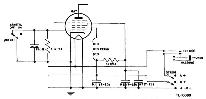
Figure 28. Frequency Meter BC-221-(1), functional diagram, crystal-oscillator circuit.
