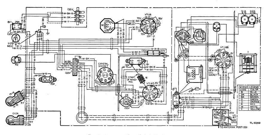
Figure 66. Frequency Meter BC-221-AC, chassis wiring diagram.
