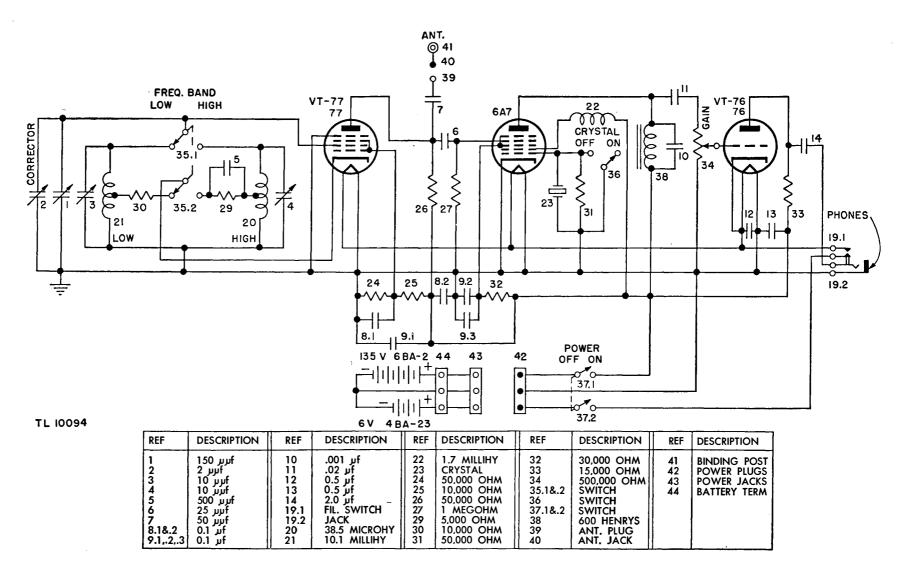
Figure 31. Frequency Meter BC-221-A, schematic diagram.
