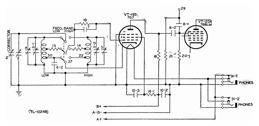
Figure 47. Frequency Meter BC-221-E, functional diagram, variable frequency oscillator circuit.
