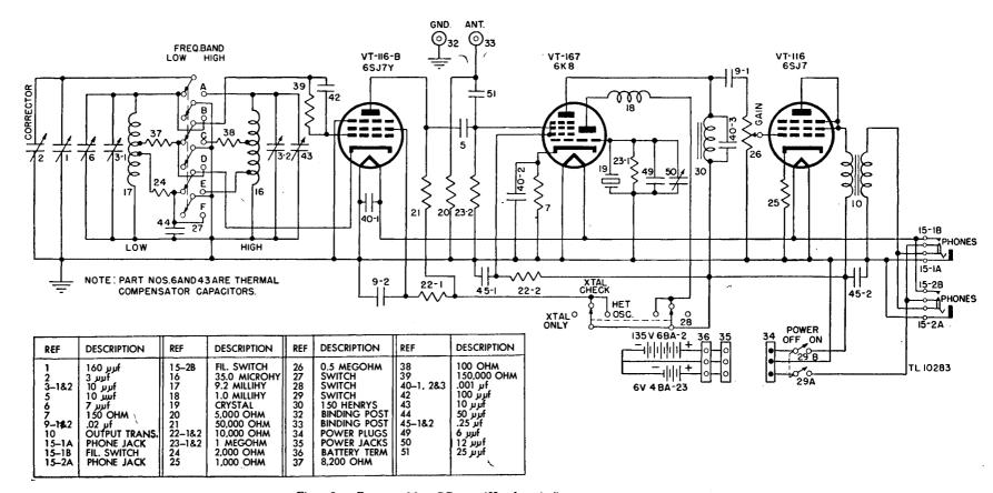
Figure 80. Frequency Meter BC-221-AH, schematic diagram.
