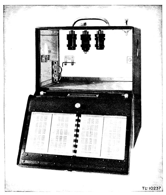
Figure 20. Frequency Meter BC-22I-B, view of cabinet interior and calibration book.
