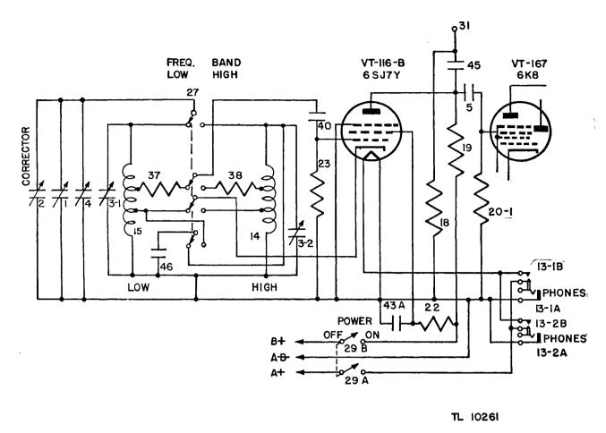
Figure 57. Frequency Meter BC-221-M, functional diagram, variable frequency oscillator circuit.
