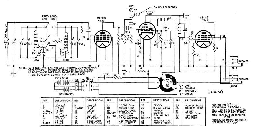
Figure 71. Frequency Meters BC-221-N and BC-221-AA, schematic diagram.
