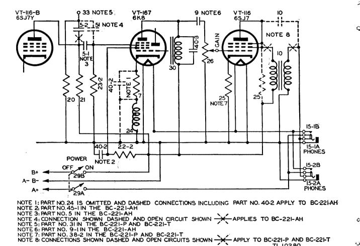
Figure 77. Frequency Meter BC-221-(6), functional diagram, detector and audio-amplifier circuits.
