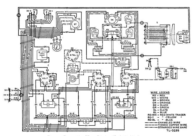
Figure 43. Frequency Meter BC-221-B (early model), chassis wiring diagram.
