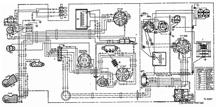
Figure 64. Frequency Meter BC-221-M, chassis wiring diagram.
