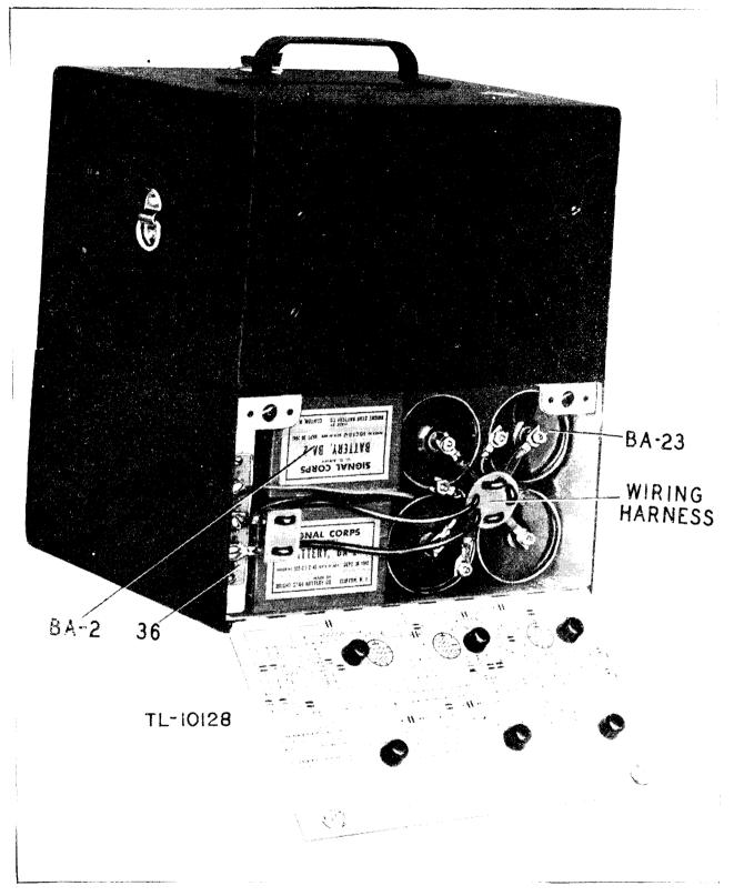
Figure 10. Use of wiring harness with buttery installation, in metal cabinet.
