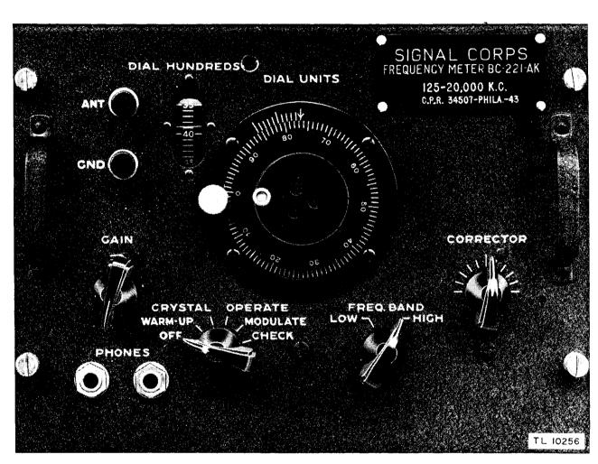
Figure 8. Frequency Meter BC-221-AK, control panel lay-out.
