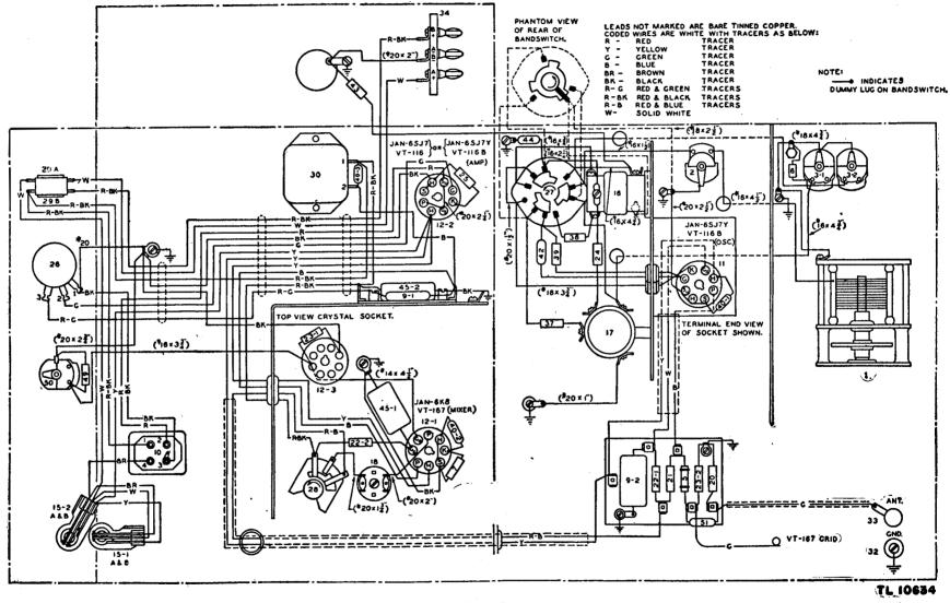
Figure 83. Frequency Meter BC-221-AH, chassis wiring diagram.
