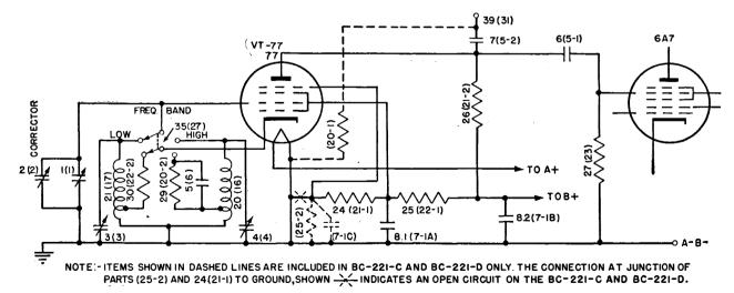
Figure 29. Frequency Meter BC-221-(1), functional diagram, variable frequency oscillator circuit.
