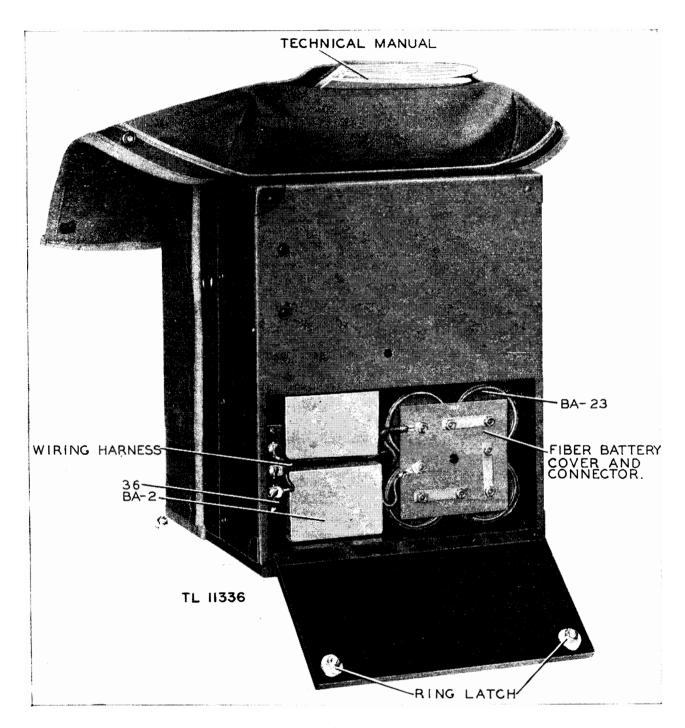
Figure 67. Frequency Meter BC-221-(3), wooden cabinet, battery installation.
