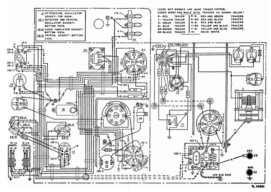
Figure 101. Frequency Meter BC-221-AJ, chassis wiring diagram.
