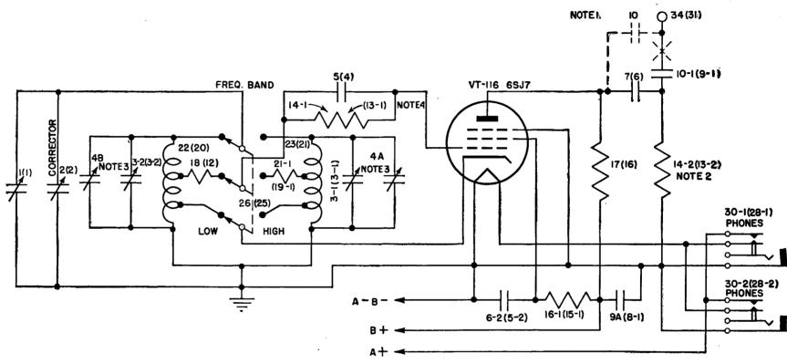
NOTE I: CONNECTION SHOWN DASHED AND OPEN CIRCUIT SHOWN APPLIES TO EARLY MODEL OF BC-221-B.
