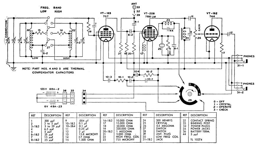
Figure 49. Frequency Meter BC-221-E, schematic diagram.
