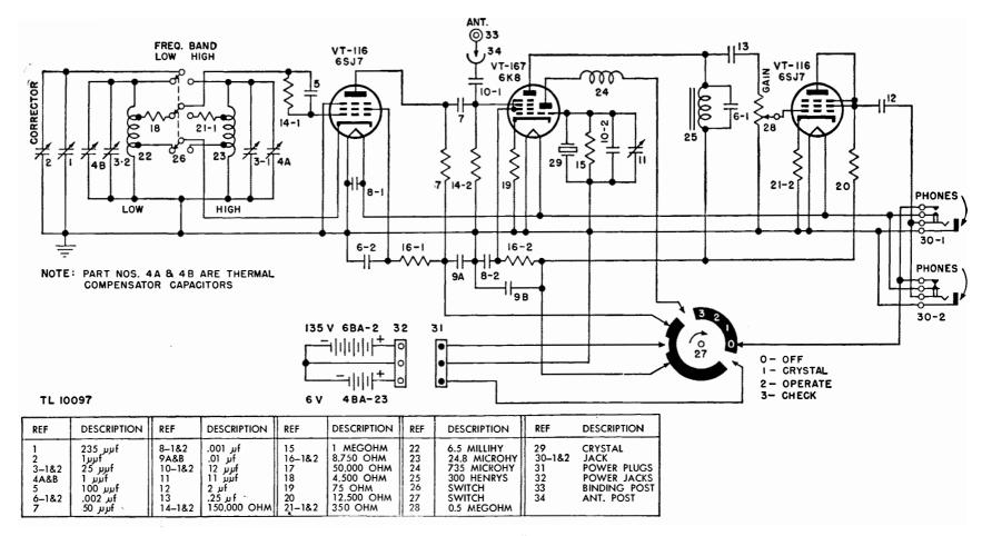
Figure 41. Frequency Meter BC-221-B (late model), schematic diagram.
