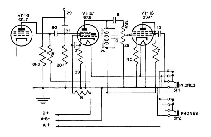
Figure 70. Frequency Meter BC-221-(5), functional diagram, detector and audio-amplifier circuits.
