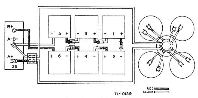
Figure 12. Battery connection details, metal cabinet.
