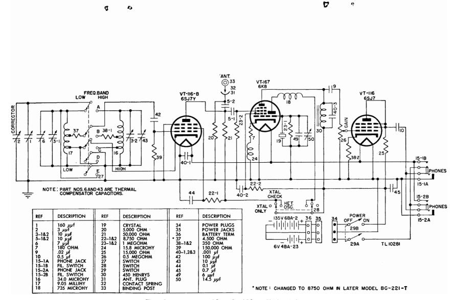
Figure 78. Frequency Meters BC-221-P and BC-221-T, schematic diagram.
