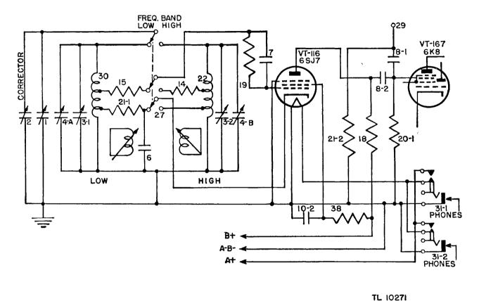
Figure 69. Frequency Meter BC-221-(5), functional diagram, variable frequency oscillator circuit.
