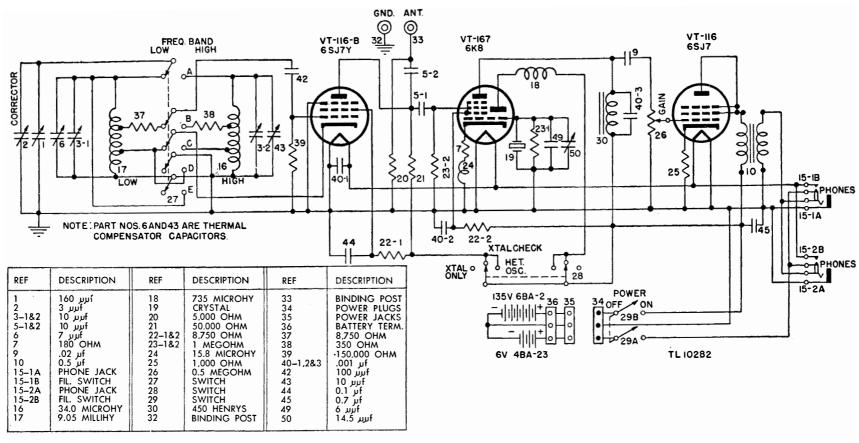
Figure 79. Frequency Meter BC-221-AF, schematic diagram.
