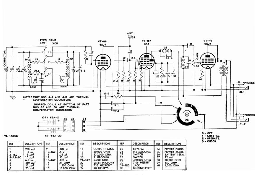
Figure 87. Frequency Meter BC-221-AE, schematic diagram.
