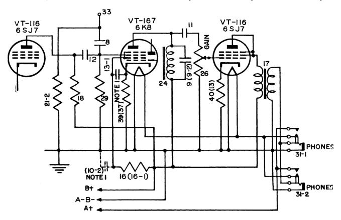
NOTE I: RART NO. 13-1 IS OMITTED & REPLACED BY PART NO. (10-2) SHOWN IN DASHED LINES, IN THE BC-221-AG.
