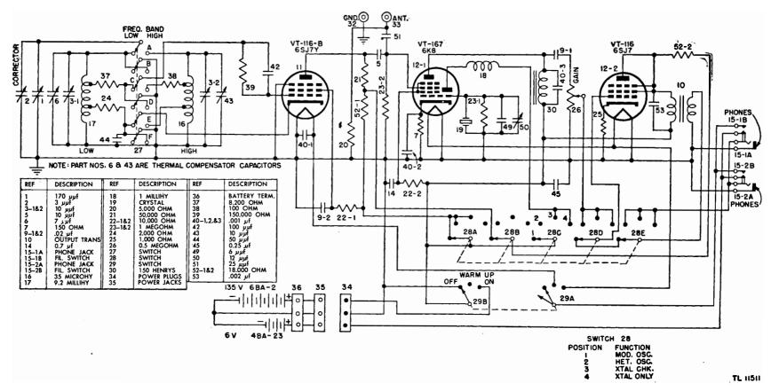
Figure 100. Frequency Meter BC-221-AL, schematic diagram.
