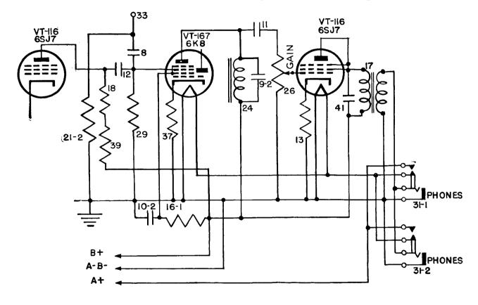
Figure 93. Frequency Meter BC-221-AK, functional diagram, detector and audio-amplifier circuits.
