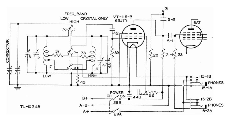
Figure 52. Frequency Meter BC-221-(3), functional diagram, variable frequency oscillator circuit.
