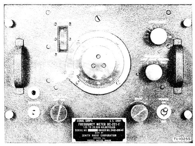
Figure 5. Frequency Meters BC 221 F, BC-221-J, BC 221 K, and BC 221 L, control penal big-out.
