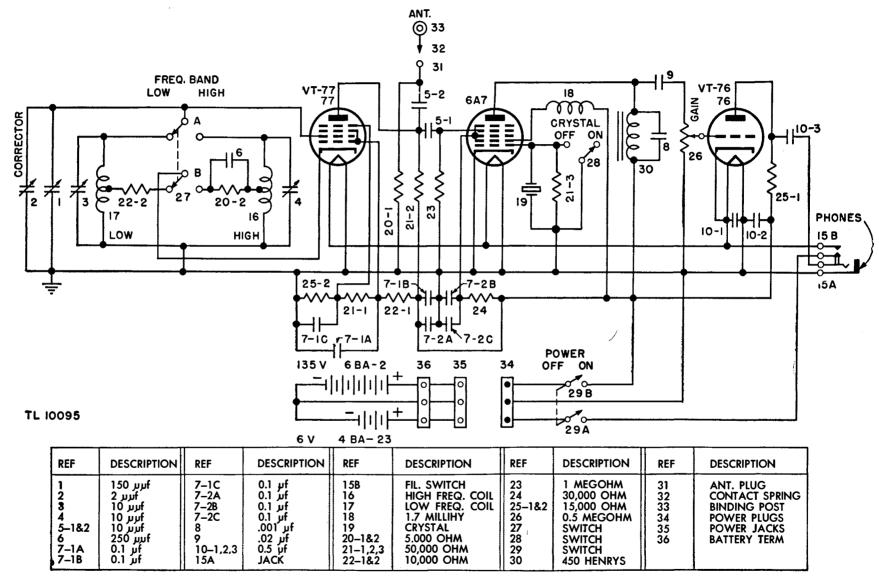
Figure 32. Frequency Meters BC-221-C and BC-221-D, schematic diagram.
