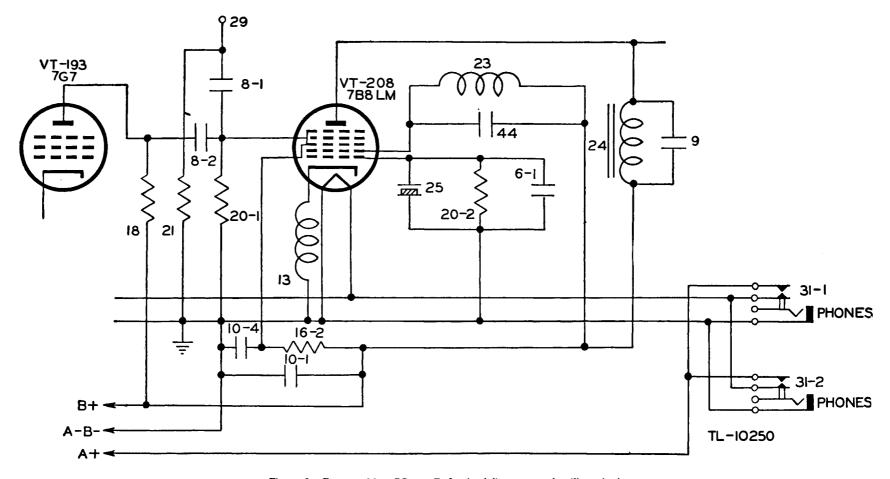
Figure 46. Frequency Meter BC-221-E, functional diagram, crystal-oscillator circuit.
