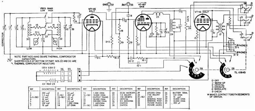
Figure 94. Frequency Meter BC-221-AK, schematic diagram.
