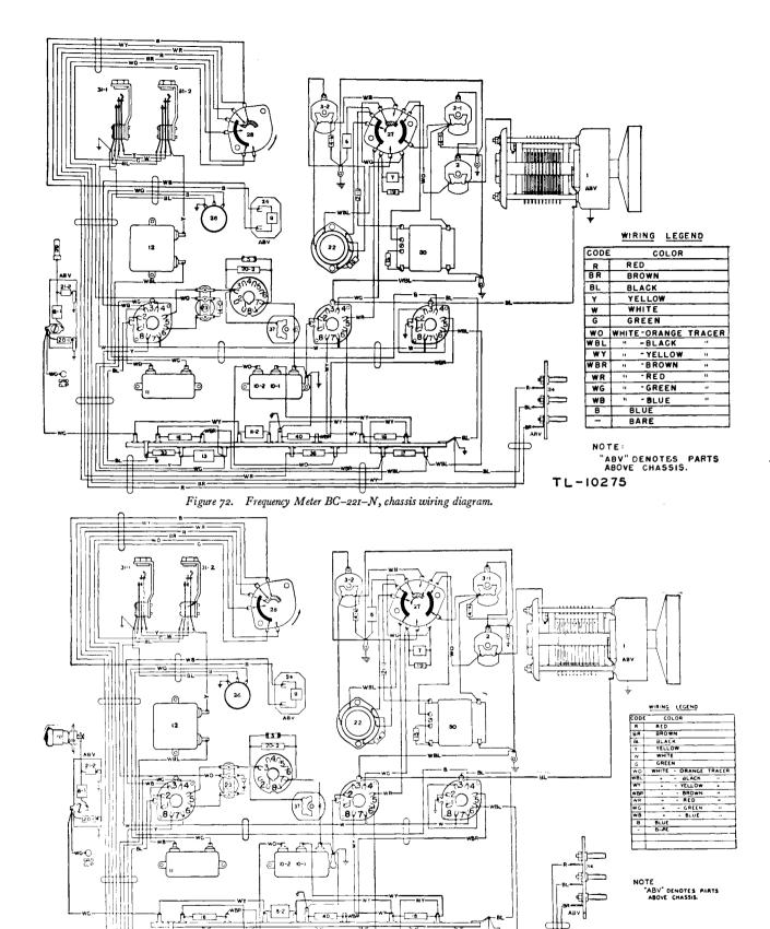
Figure 73. Frequency Meter BC-221-AA, chassis wiring diagram.
