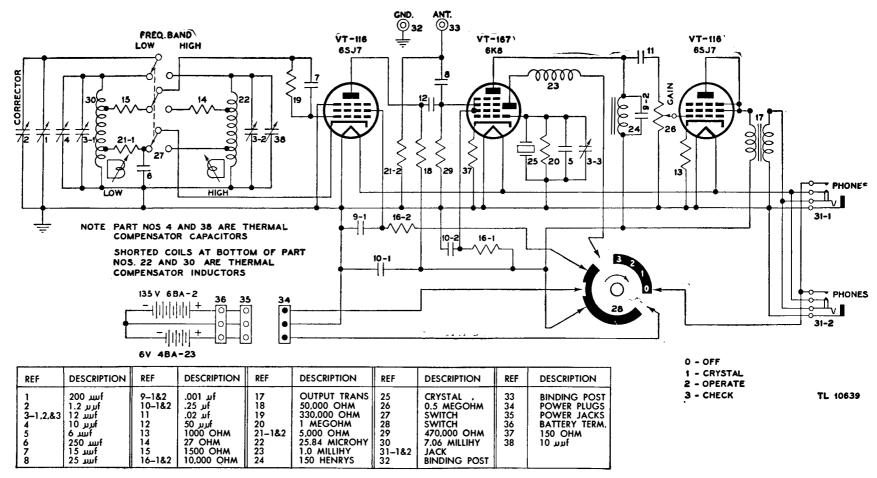
Figure 88. Frequency Meter BC-221-AG, schematic diagram.
