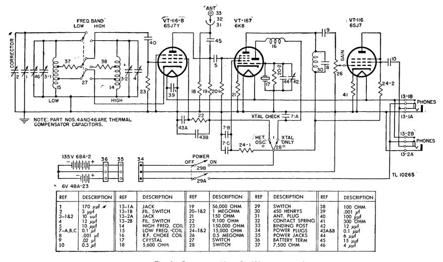
Figure 62. Frequency Meters BC-221-O and BC-221-R, schematic diagram.
