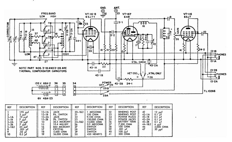
Figure 63. Frequency Meter BC-221-AC, schematic diagram.
