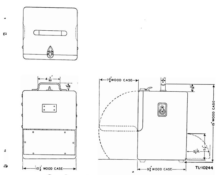
Figure 27. Frequency Meter BC-221-(&), typical dimensions, wooden cabinet (subject to slight variations).
