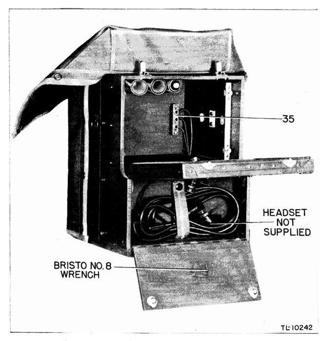
Figure 25. Frequency Meter BC-221-( $\mathcal{E}$ ), typical wooden cabinet, showing headset compartment.
