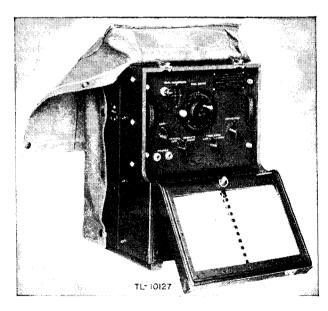
Figure 2. Frequency Meter BC-221-( $\mathscr{C}$ ), in wooden cabinet.
