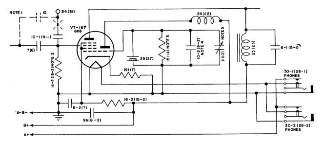
NOTE 1:- CONNECTION SHOWN DASHED AND OPEN CIRCUIT SHOWN APPLIES TO EARLY MODEL OF BC-221-B NOTE 3:- PART NO.15-1 IN EARLY MODEL OF BC-221-B
