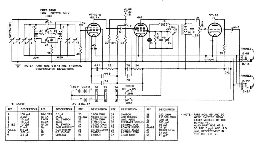
Figure 54. Frequency Meter BC-221-(3), schematic diagram.
