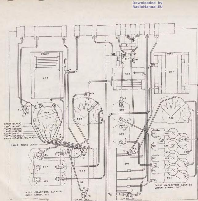
NOTE FOR SOLDERING :-WIRE TO BE FASTENED MECHANICALLY TO TERMINALS BEFORE SOLDERING. USE ROSIN CORE SOLDER B20 D3C.
