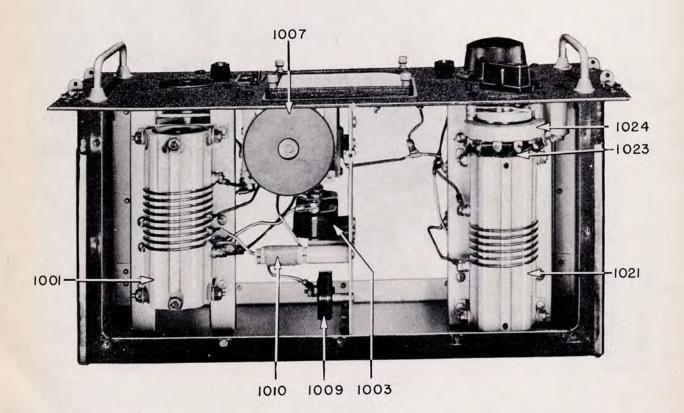
FIG. 40. TRANSMITTER TUNING UNIT TU-10-B, BOTTOM VIEW, COVER REMOVED
