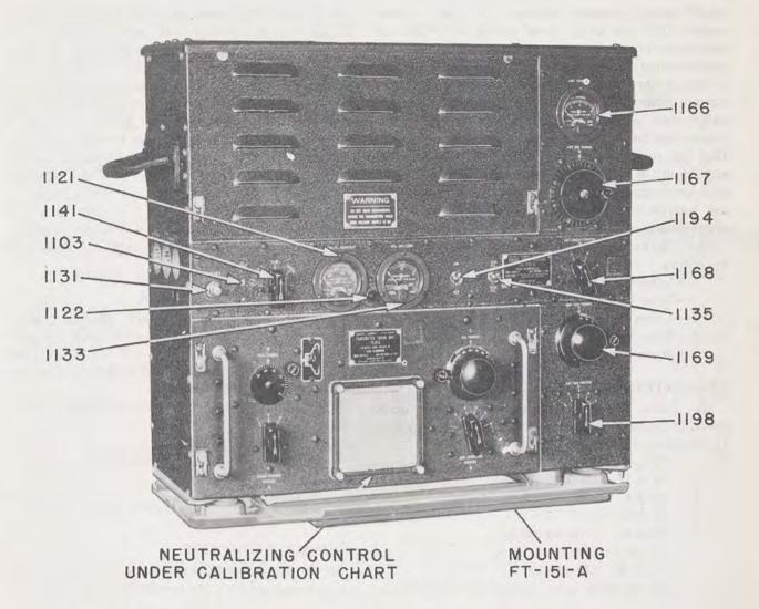
FIG. 5. RADIO TRANSMITTER BC-375-D, TRANSMITTER TUNING UNIT TU-22-B IN PLACE
