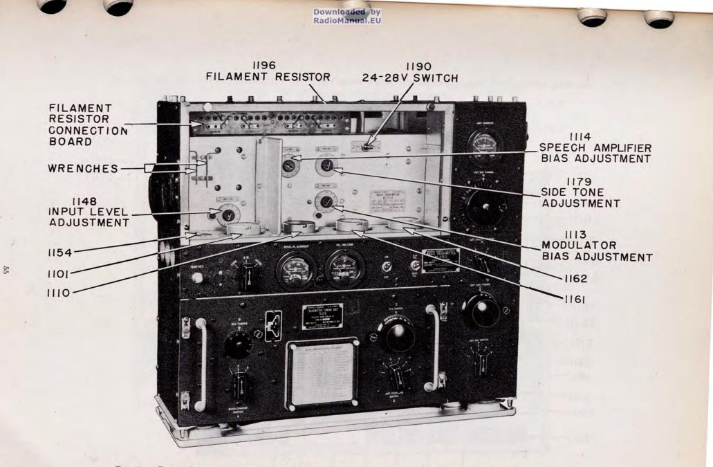
FIG. 25. RADIO TRANSMITTER BC-375-D, TUBE COMPARTMENT SHIELD AND TOP COVER OFF AND TRANS-MITTER TUNING UNIT IN PLACE
