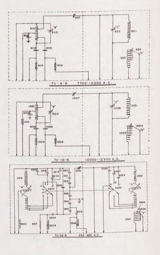
FIG. 52. TRANSMITTER TUNING UNITS, SCHEMATIC DIAGRAM
