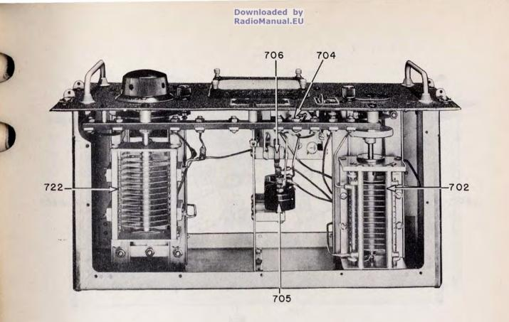
FIG. 33. TRANSMITTER TUNING UNIT TU-7-B, TOP VIEW, COVER REMOVED
