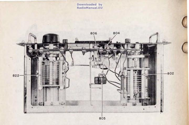
FIG. 35. TRANSMITTER TUNING UNIT TU-8-B, TOP VIEW, COVER REMOVED
