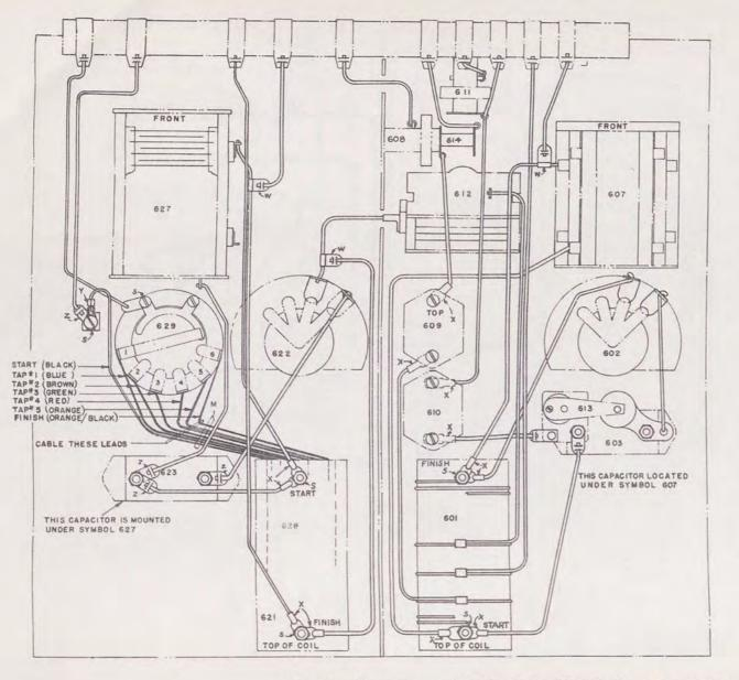
NOTE: THERE SHALL BE NO SHARP POINTS LEFT AFTER UNIT IS WIRED EITHER FROM LUMPS OF SOLDER OR IRREGULARLY CUT WIRE ENDS. WIRE TO BE FASTENED MECHANICALLY TO TERMINALS BEFORE SOLDERING. USE ROSIN CORE SOLDER B2003C
