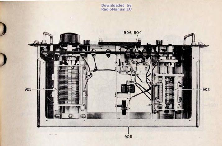
FIG. 37. TRANSMITTER TUNING UNIT TU-9-B, TOP VIEW, COVER REMOVED
