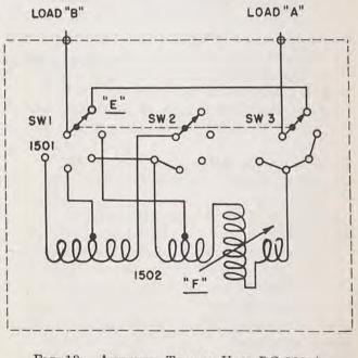
FIG. 19. ANTENNA TUNING UNIT BC-306-A, Schematic Diagram
