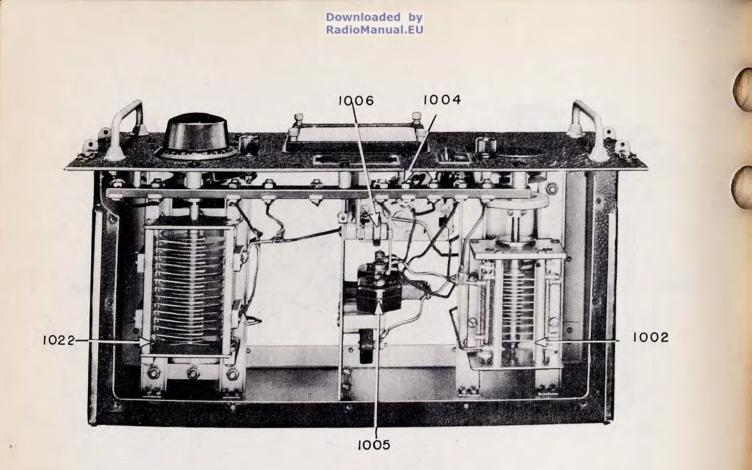
FIG. 39. TRANSMITTER TUNING UNIT TU-10-B, TOP VIEW, COVER REMOVED
