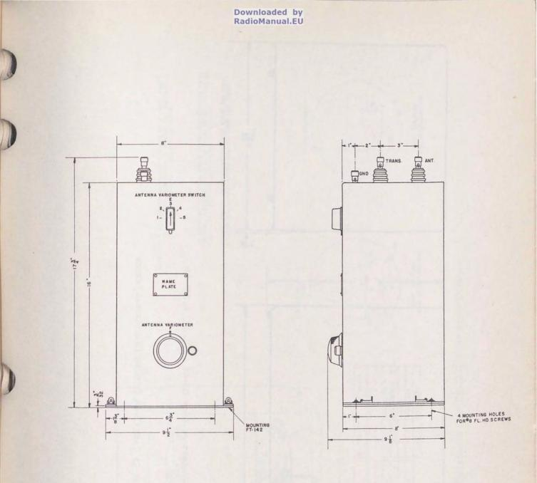
Weight of Antenna Tuning Unit BC-306-A Less Mounting ..... 9.062 lb Weight of Mounting FT-142 ..... 0.687 lb
