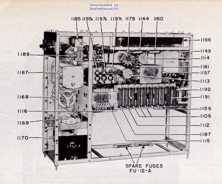
FIG. 26. RADIO TRANSMITTER BC-375-D, REAR VIEW, MOUNTING FT-151-A AND SHIELDS REMOVED
