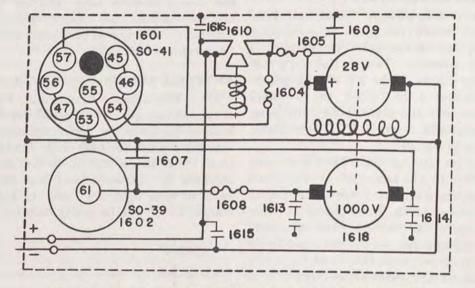
FIG. 20. DYNAMOTOR UNIT PE-73-C, SCHEMATIC DIAGRAM
