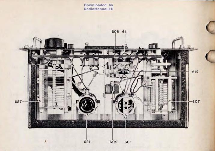
FIG. 31. TRANSMITTER TUNING UNIT TU-6-B, TOP VIEW, COVER REMOVED
