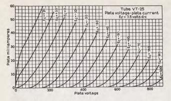
FIG. 18. TUBE VT-25, CHARACTERISTIC CURVES
