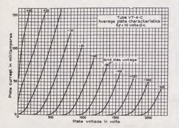
FIG. 17. TUBE VT-4-C, CHARACTERISTIC CURVES
