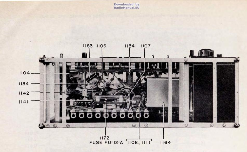
FIG. 28. RADIO TRANSMITTER BC-375-D, BOTTOM VIEW, MOUNTING FT-151-A AND SHIELDS REMOVED
