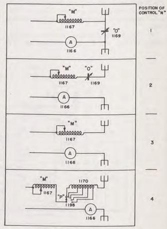
FIG. 12. RADIO TRANSMITTER BC-375-D, FUNCTIONAL DIAGRAM OF ANTENNA TUNING CIRCUITS
