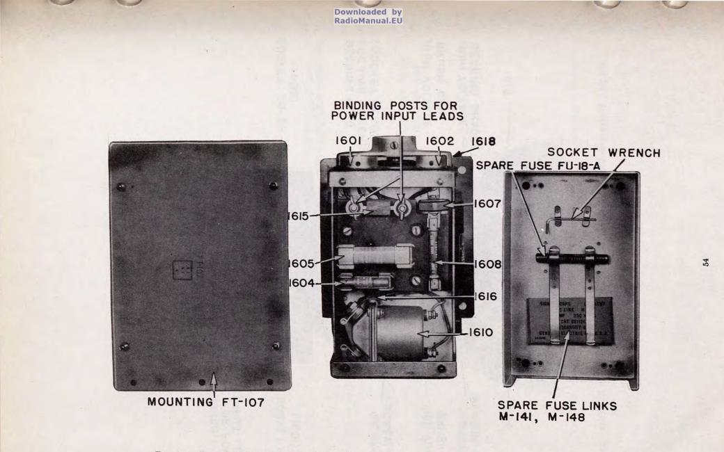
FIG. 24. DYNAMOTOR UNIT PE-73-C, TOP VIEW, MOUNTING FT-107 AND RELAY-FUSE BOX COVER Removed
