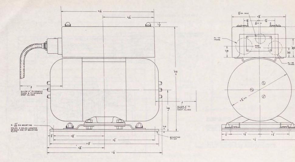
Weight of Dynamotor Unit PE-73-C Less Mounting ..... 37.25 1b Weight of Mounting FT-107 ..... 1.45 lb
