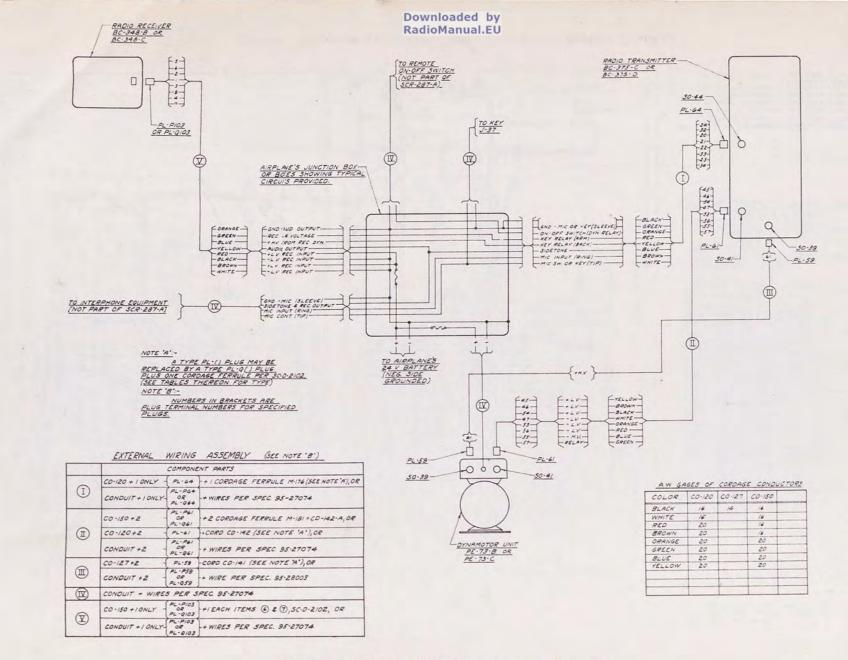
FIG. 60. RADIO SET SCR-287-A, CORDING DIAGRAM
