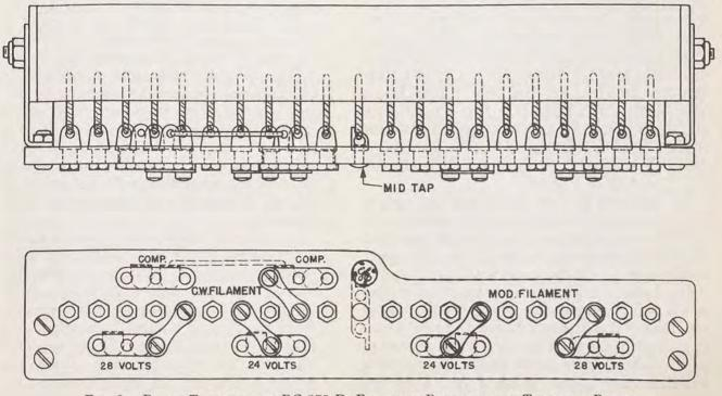
FIG. 9. RADIO TRANSMITTER BC-375-D, FILAMENT RESISTOR AND TERMINAL BOARD
