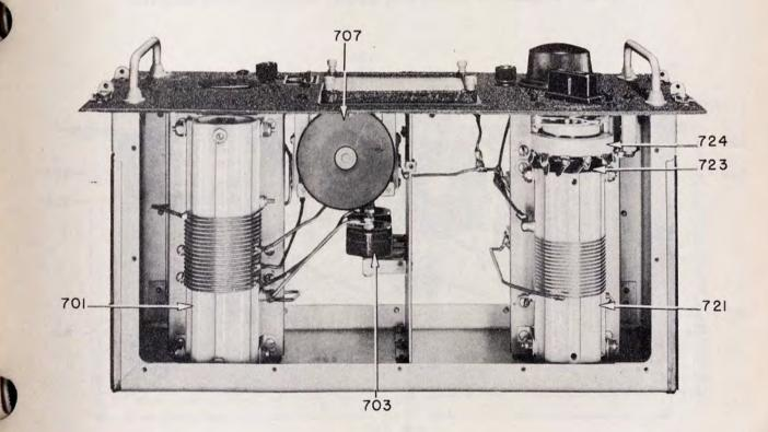
FIG. 34. TRANSMITTER TUNING UNIT TU-7-B, BOTTOM VIEW, COVER REMOVED
