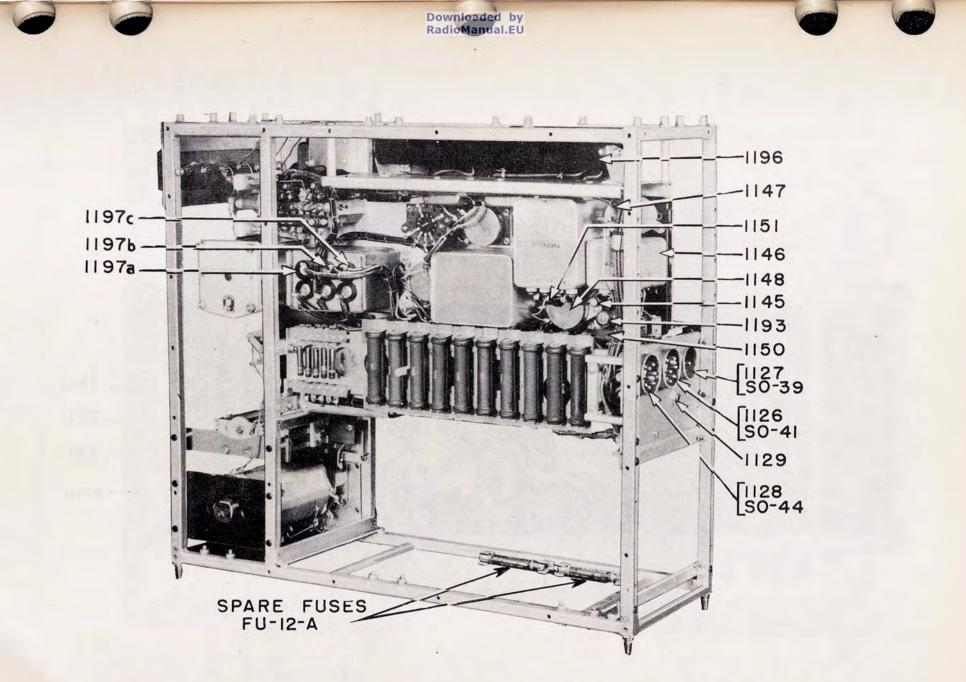
FIG. 27. RADIO TRANSMITTER BC-375-D, REAR VIEW, MOUNTING FT-151-A AND SHIELDS REMOVED
