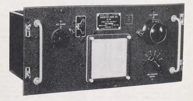
Fig. 6. TYPICAL FRONT VIEW OF A TRANSMITTER TUNING UNIT WITHOUT A BAND CHANGE SWITCH
