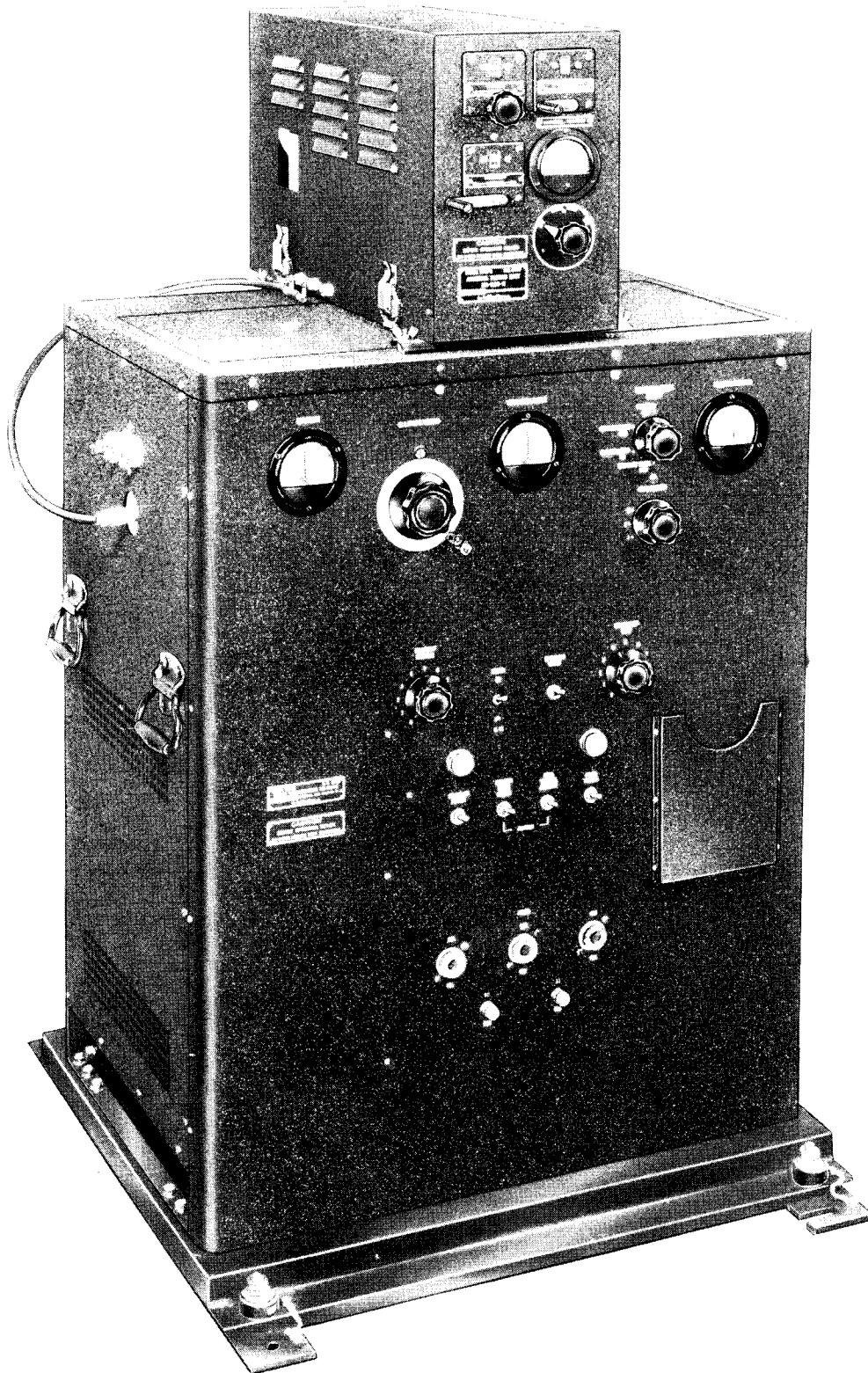
Figure 1. Radio Transmitter BC-610 I with Antenna Tuning Unit BC-939-B in position.
