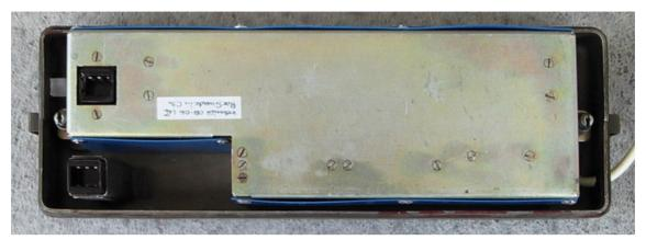
This shows the power supply in its metal case and installed in the battery box.
