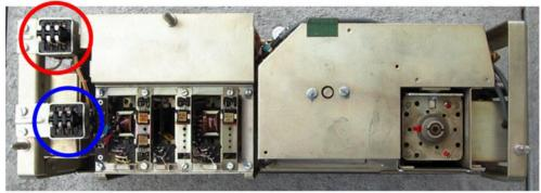
St2: batteries i/p, fil 1.2V 1(-) and 5(+), 7.2V 6(-) and 4(+), 2 and 3 n/c, 5 and 6 via St1 to Sch1, 1 to gnd, 4 to gnd at DC/DC converter
