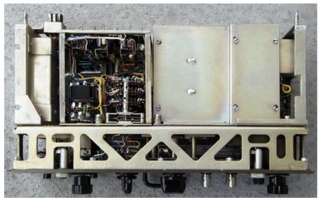
Bottom view, audio circuits and mode and power switches on the left
