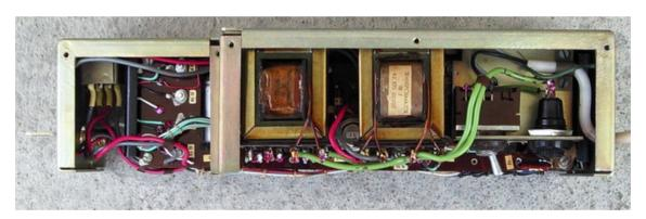
View from the top and bottom, note Zá1 on the left, new capacitors have been fitted
