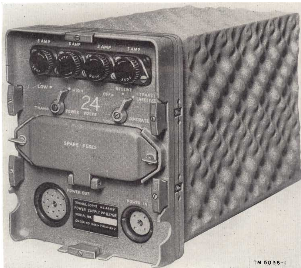
Figure 1. Power supply PP-112/GR.
