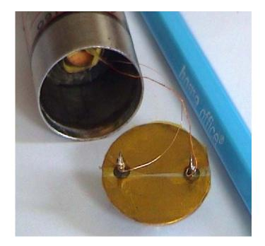
Then carefully connect the wires to the tags.
