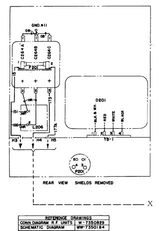
Connection Diagram, Type CG-46116 Receiver Unit No. 2
