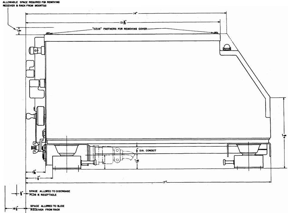
Outline Drawing of Single Receiver, Model RAX-1 Radio Receiving Equipment
