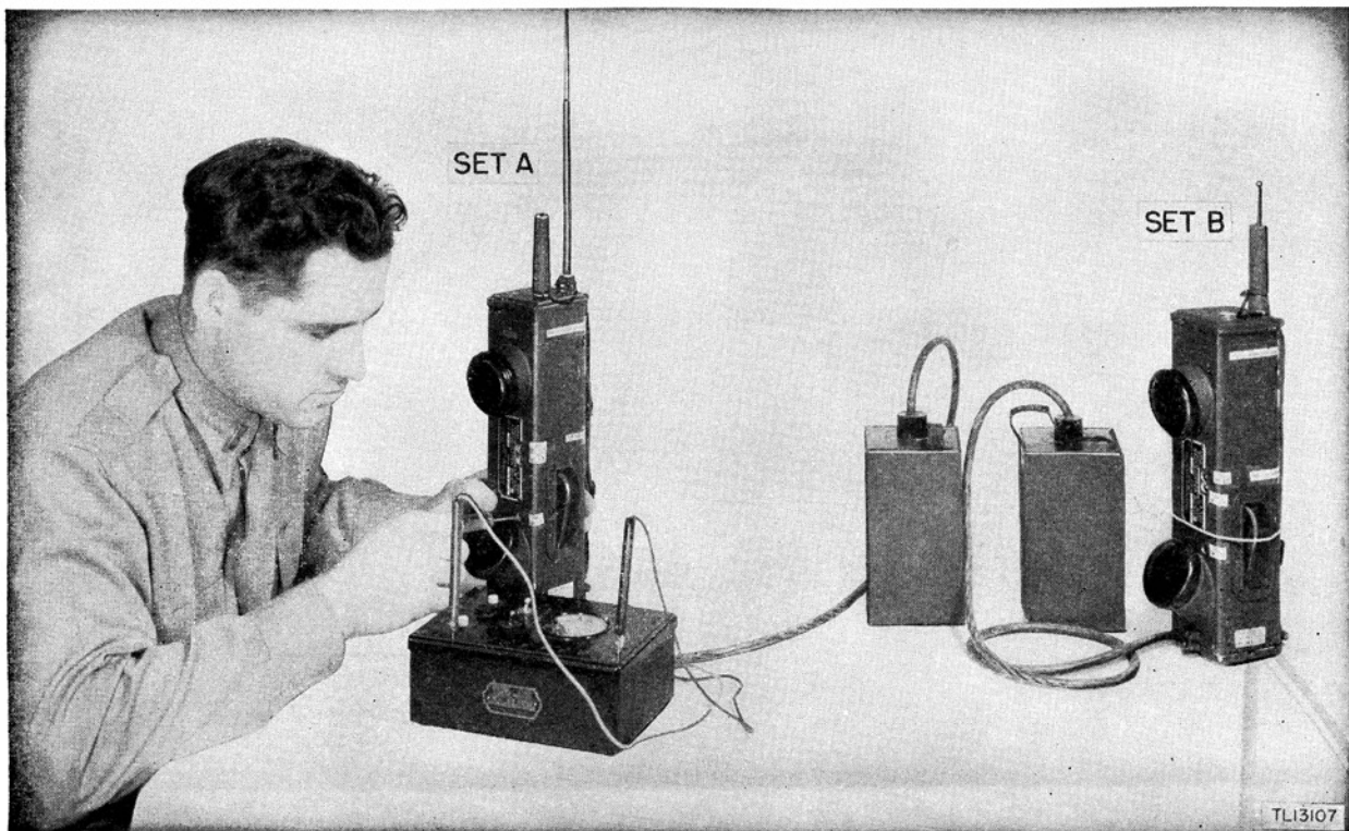
Figure 84. Emergency test equipment, using milliammeter.
