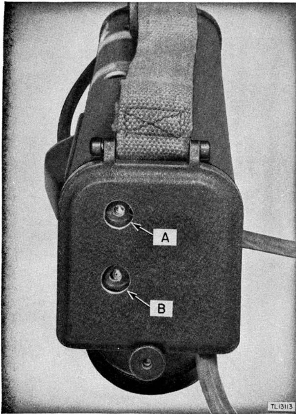
Figure 77. Battery check holes.
