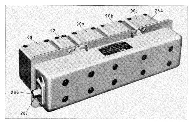
FIGURE 10—COIL UNIT C-439 (DUAL, RECEIVING)
