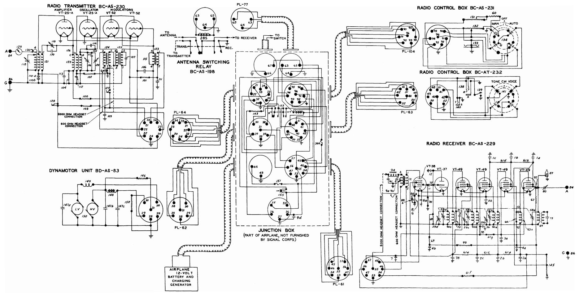
FIGURE 19-RADIO SET SCR-AS-183, SCHEMATIC CIRCUIT DIAGRAM
