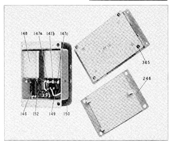
FIGURE 8-DYNAMOTOR UNIT BD-AS-83, BOTTOM VIEW
