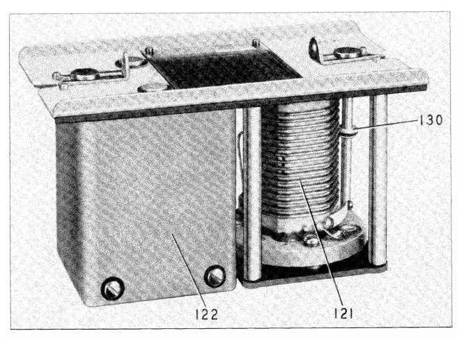
FIGURE 16—COIL SET C-435 (TRANSMITTING)
