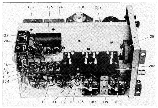
FIGURE 13—RADIO TRANSMITTER BC-AS-230, BOTTOM VIEW
