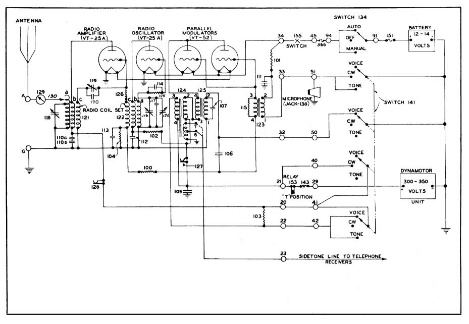
FIGURE 18—RADIO TRANSMITTER BC-AS-230, FUNCTIONAL DIAGRAM
