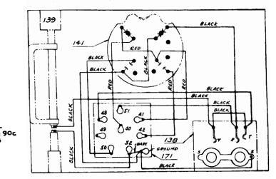
ANTENNA SWITCHING RELAY BC-AS-198
