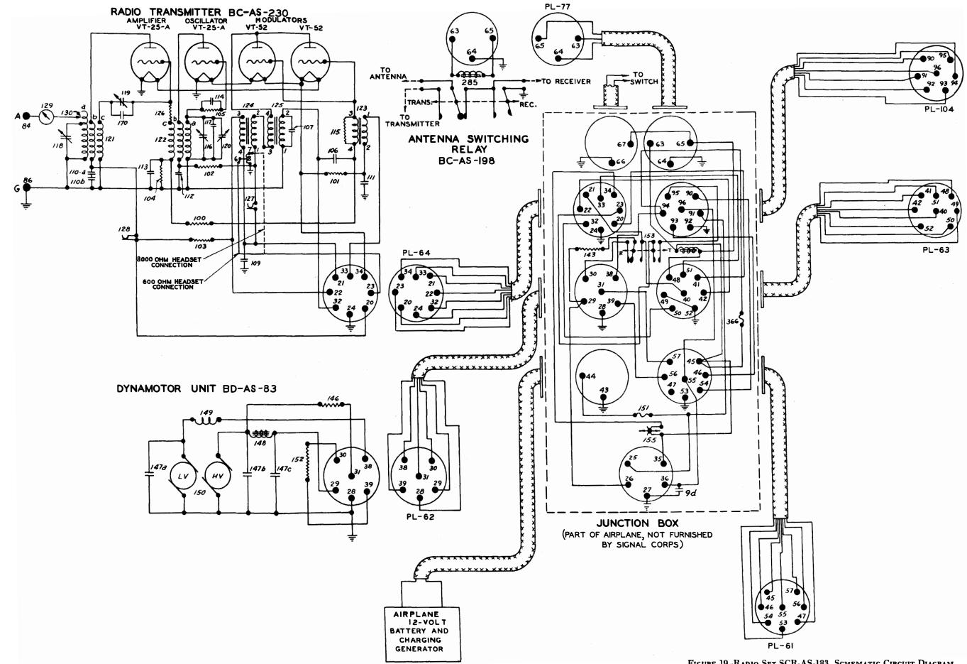
FIGURE 19-RADIO SET SCR-AS-183, SCHEMATIC CIRCUIT DIAGRAM 65
