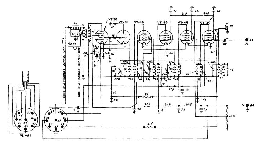
FIGURE 19-RADIO SET SCR-AS-183, SCHEMATIC CIRCUIT DIAGRAM 65A
