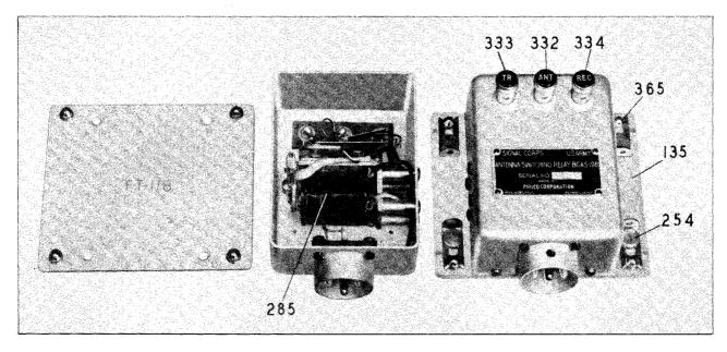
FIGURE 9—ANTENNA SWITCHING RELAY BC-AS-198
