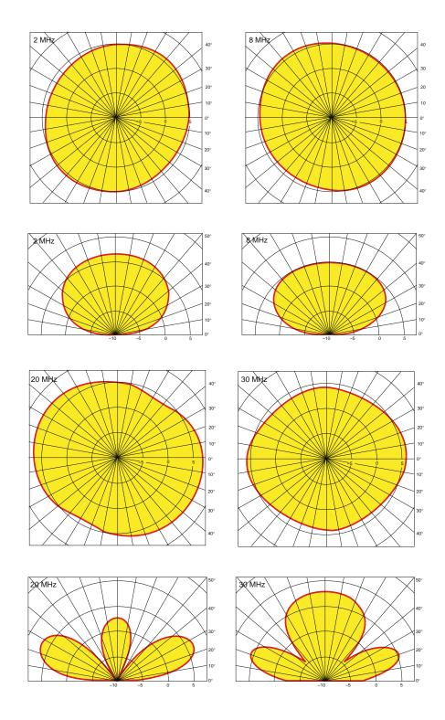
→ Azimuth and Elevation Patterns (Azimuth pattern at elevation angle of beam maximum) gain in dBi
