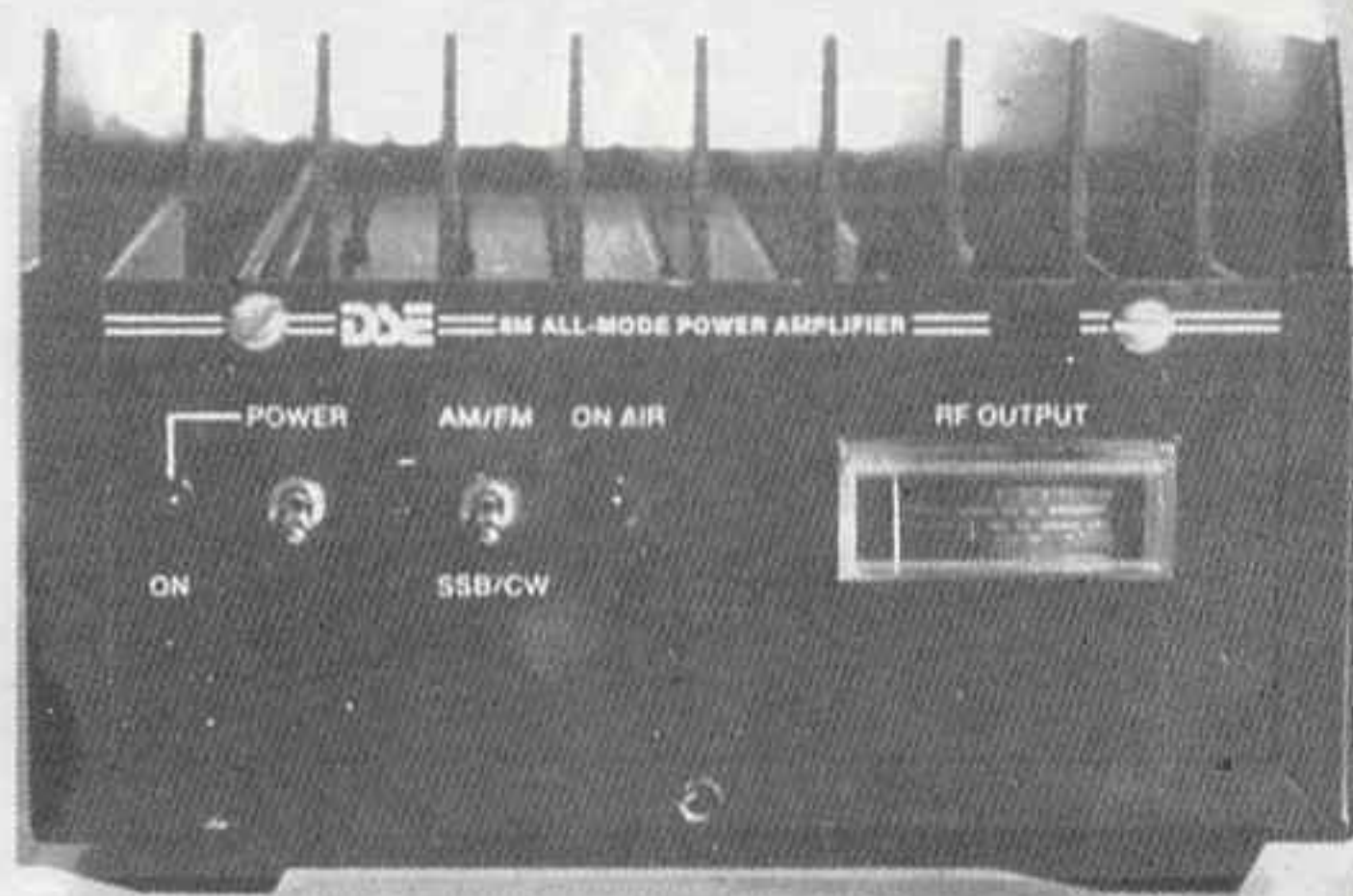
Styling of the 6m all-mode amp matches that of the 2m and 70 cm amps, with a topside heatsink and folded aluminium housing. The front panel meter indicates relative power output.
