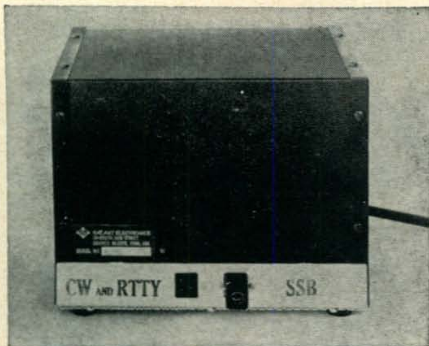
Power Supply for the Galaxy 2000+. The jumper plug is in the s.s.b. position.
