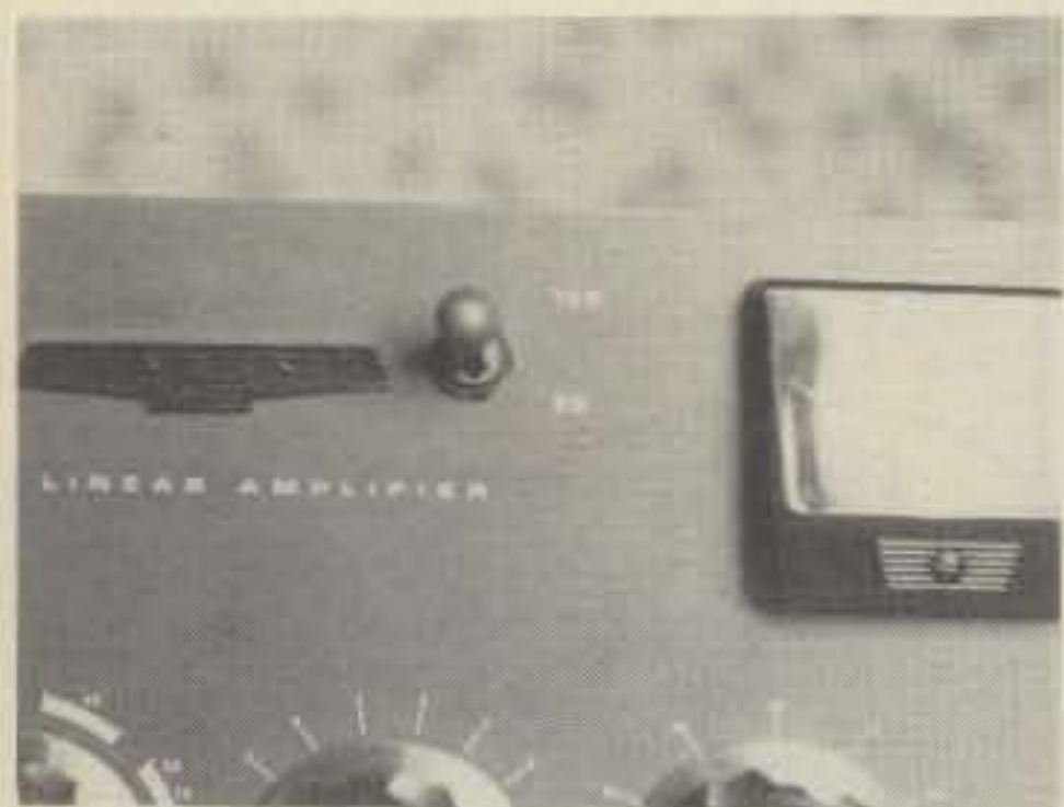
Left: The panel position of the added toggle switch. Right: Note the addition of the "160" decal.
