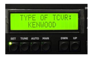
**For communication with TCVRs**, that are not supported by OM2500A as for example JST-245 and older types of Kenwood an external IF-232 converter is to be used. You can use universal products of microHAM <a href="https://www.microham.com">https://www.microham.com</a> as MKII, MK2R+ etc., which process information about the frequency in ICOM format through the CI-V output. Then the PA will be connected in the following configuration:
