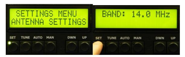
Then we select how many antennas we want per current band (1 or 2) always confirm your selection by pressing SET. The by scrolling UP / DWN you assign which PORT is used on your external antennas switch for this particular antennas. (ANT 1 ON PORT 01)
