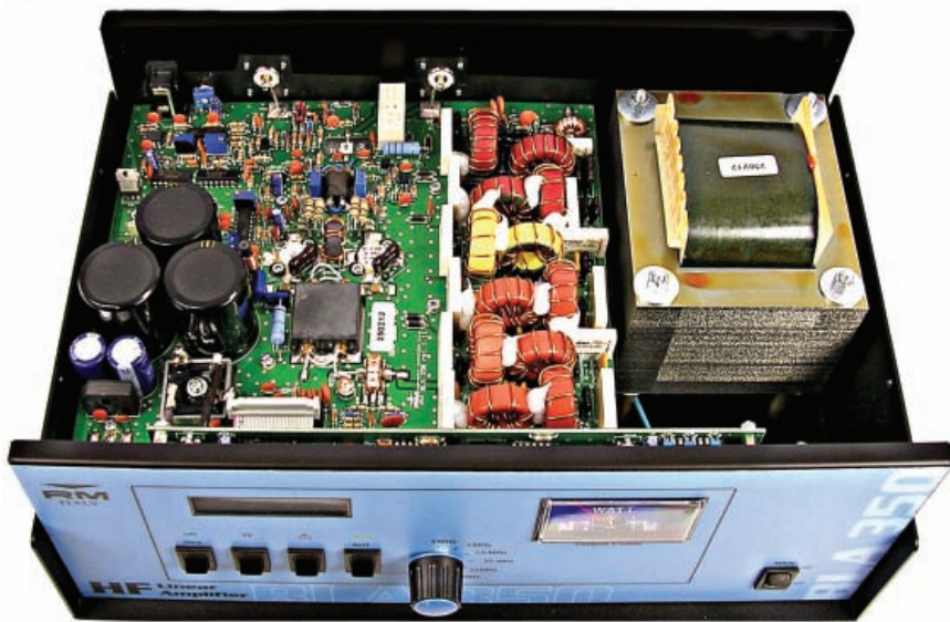
Fig. 3: There's one main printed circuit board (p.c.b.) housing the two m.o.s.f.e.t.s and a very large heat sink underneath.
