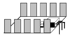
40. Mount the transistors and heatsinks to the PC board using the 4-40 screws and nuts. Solder all transistor leads. Note that the heatsinks may look slightly different from the ones shown.
