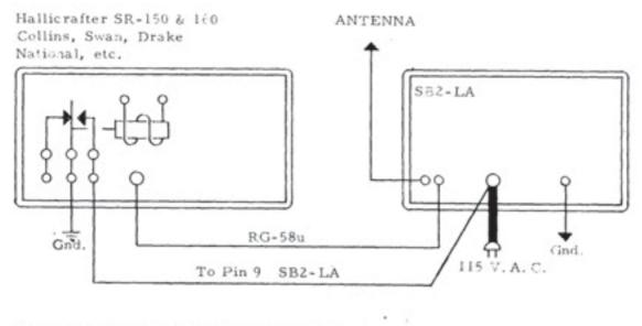
CONNECTING SB2-LA TO TRANSCEIVER OF OTHER MANUFACTURE
