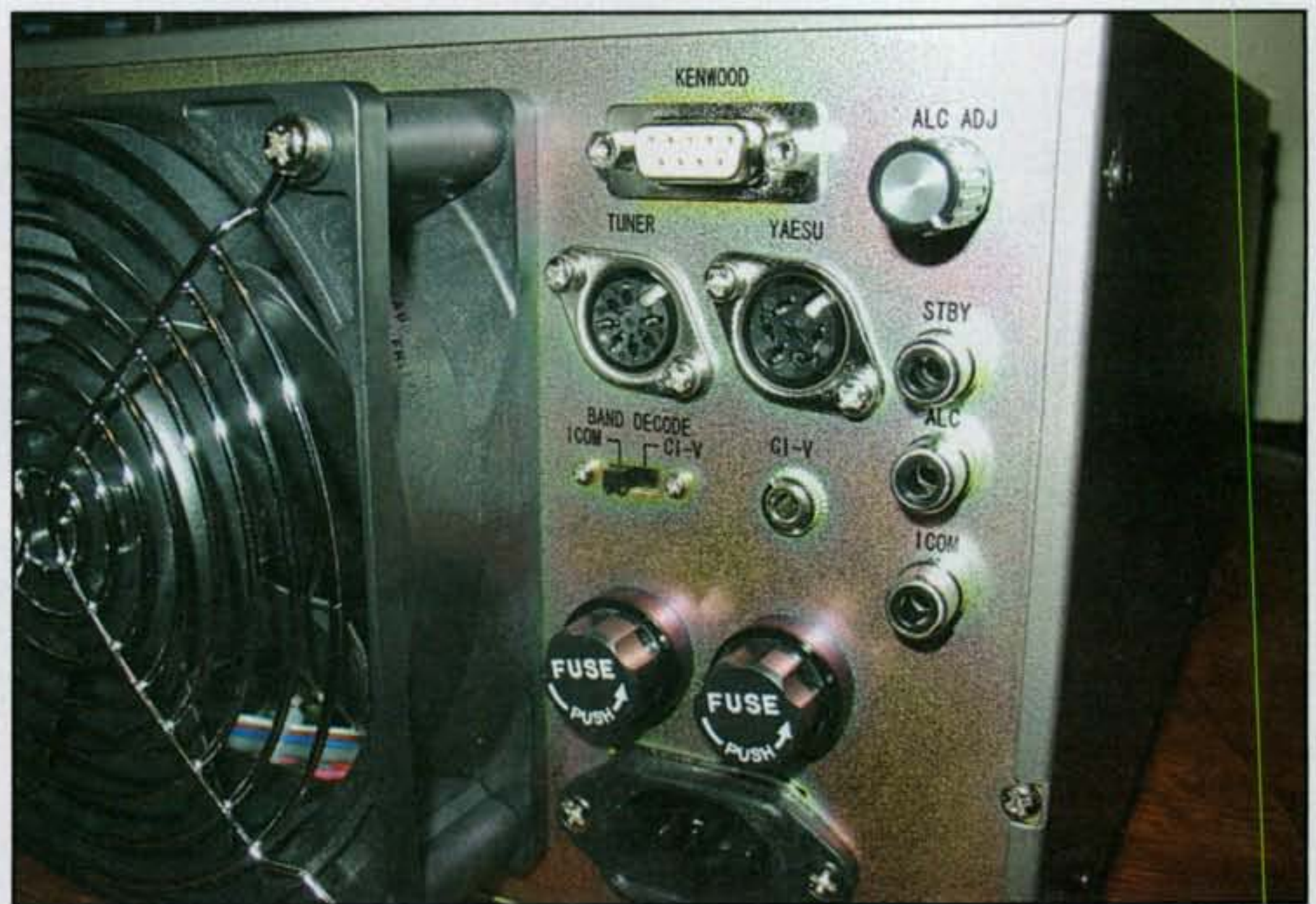
Photo D— Close-up of the well-marked transceiver interface connectors. All cables are supplied for directly interfacing band-data information from many ICOM, Kenwood, and Yaesu transceivers.
