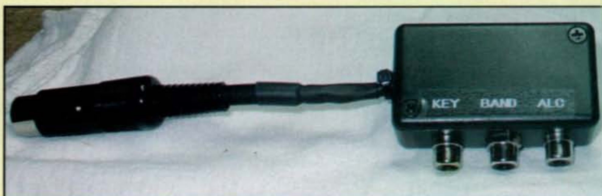
Photo F— Outside view of the IC-706MkIIIG interface.
