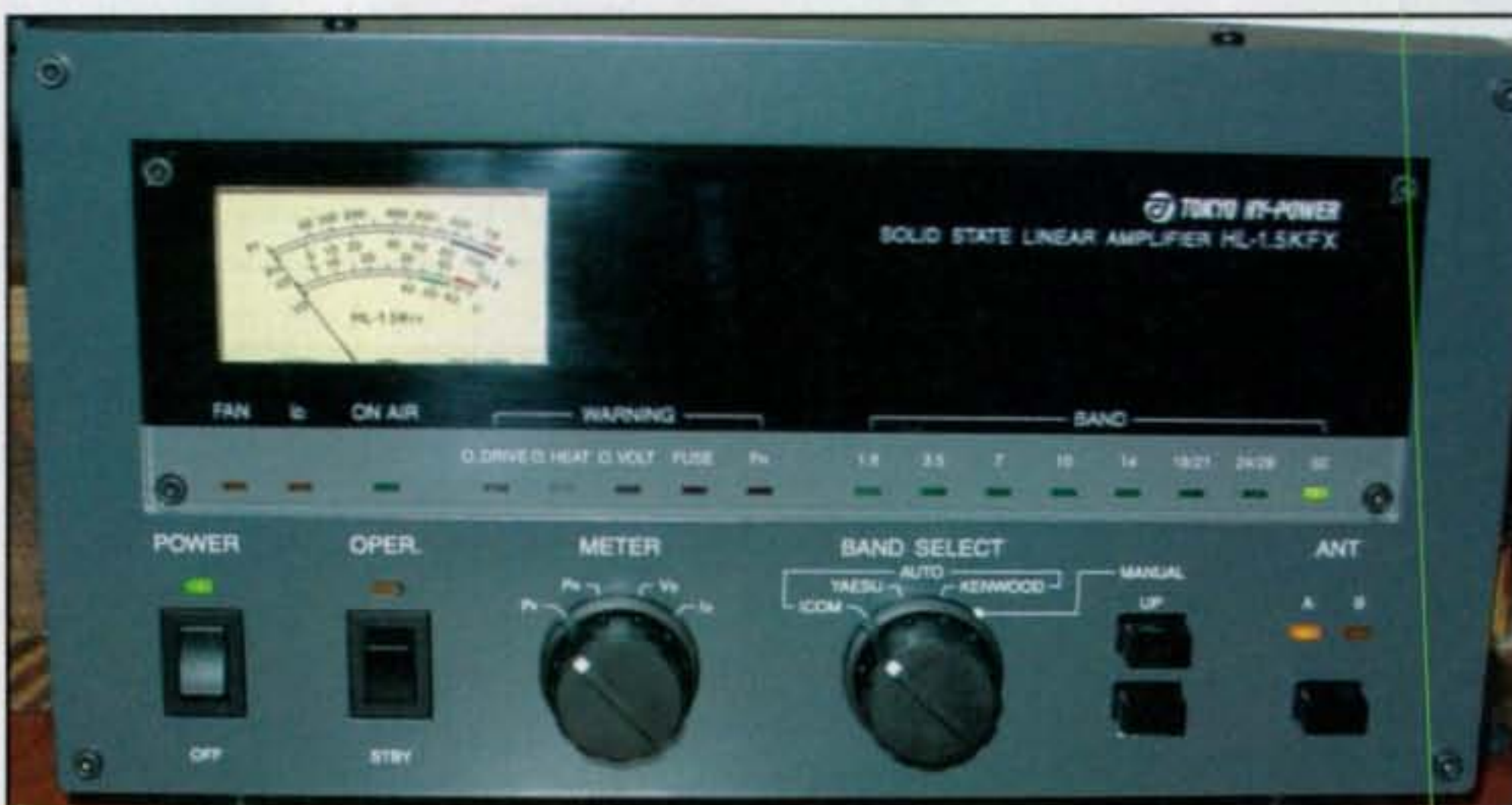
Photo A— The Tokyo Hy-Power HL-1.5KFX provides 1000 watts of power from 1.8–30 MHz and 600 watts on 6 meters.
