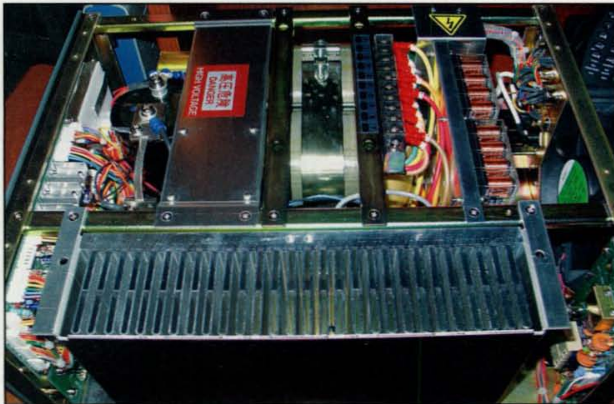
Photo B— Inside view of the amplifier. Note the massive heatsink in the foreground.
