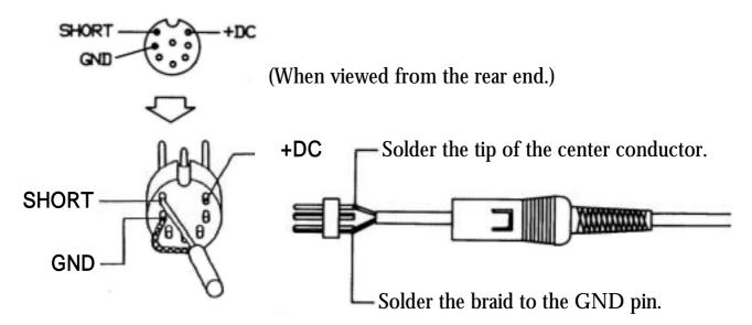
\*Note: If the transceiver externally supplies no voltage (0V, =TX Gnd.) during the TX, solder the center conductor to Pin (SHORT), or if it supplies the positive DC voltage of 2 to 15 V, then solder to Pin (+DC).
