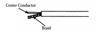
c) Peel off the sheath of the center wire tip.
