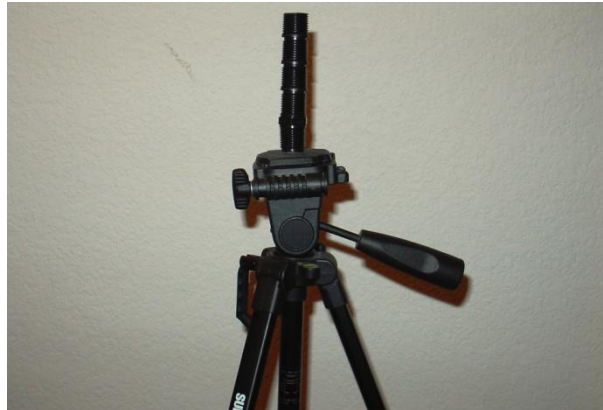
Figure 4: Camera Tripod Adapter for WalkHam Figure 5: Tripod Adapter on camera tripod
