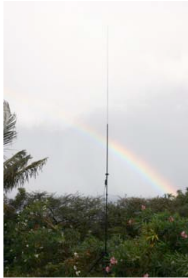
Ground mounted vertical antenna for 17m on VP2M
