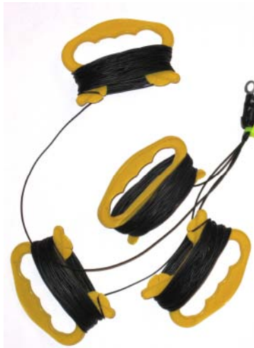
Four radial wires terminating in a single ring connector. (Assembly made by the author.)
