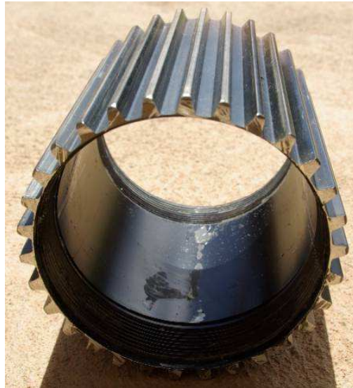
Image 7 – Threaded aluminium sleeve.
