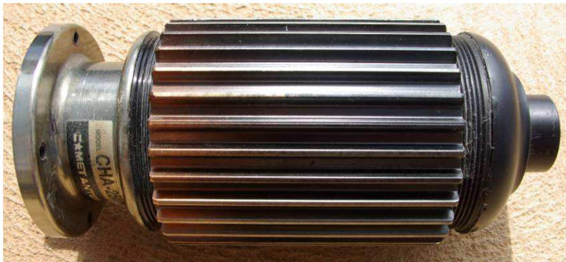
Image 3 – Showing how the top and bottom sections are screwed in.
