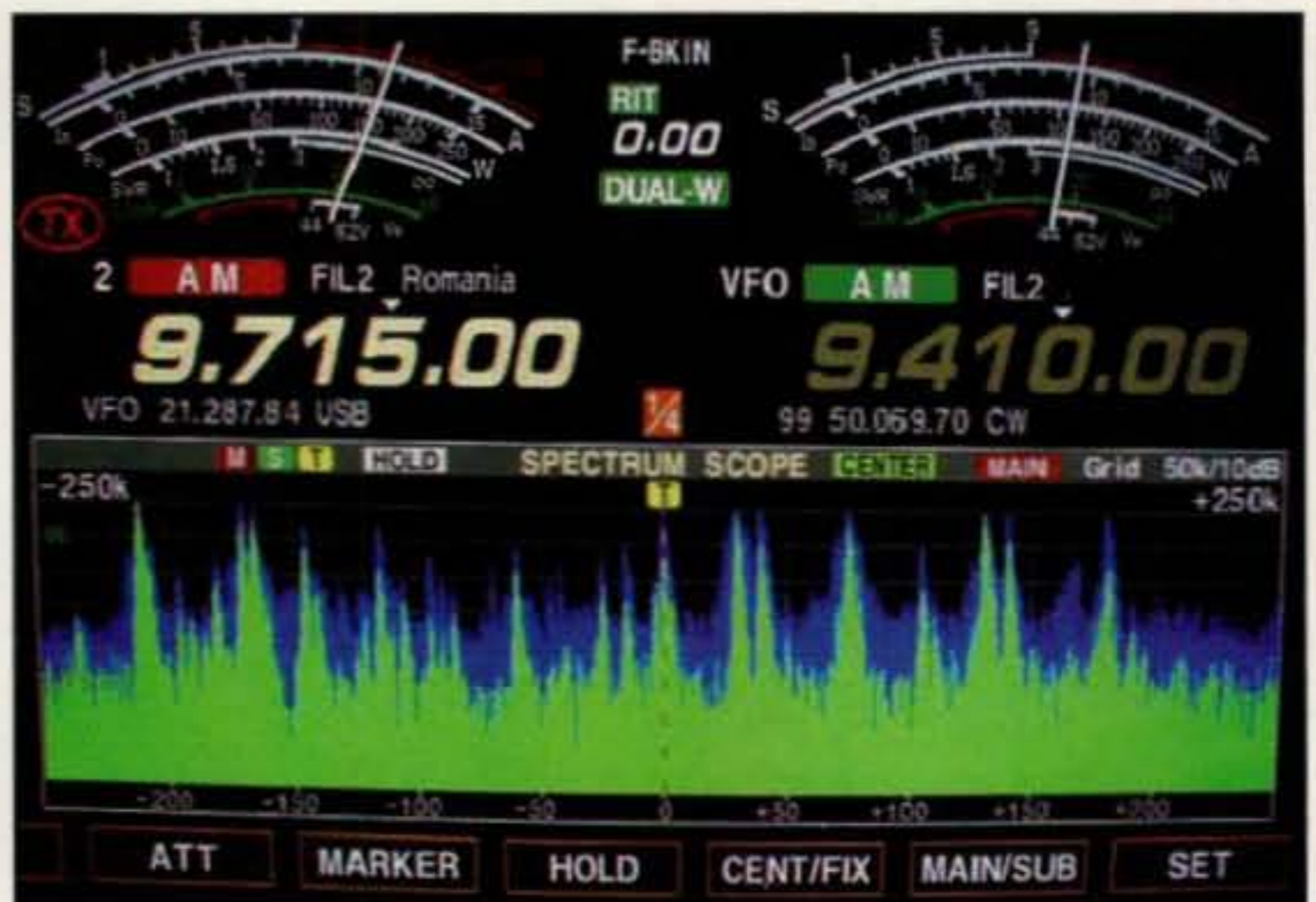
Photo E— A snapshot of the 31-meter shortwave broadcast band. The frequency range displayed is 9.465 to 9.965 MHz. Plenty of strong signals to listen to here!
