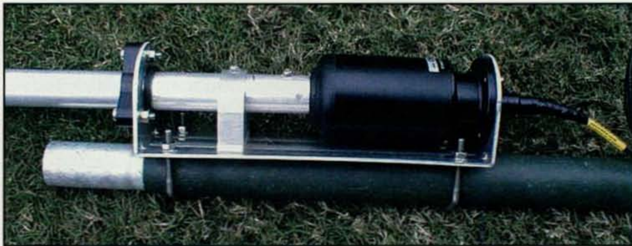
Photo B— Here is the base of the antenna mounted to an aluminum mast section. Notice the exceptionally small matching network (black cylindrical section) of the antenna. No extended radials; this is it!
