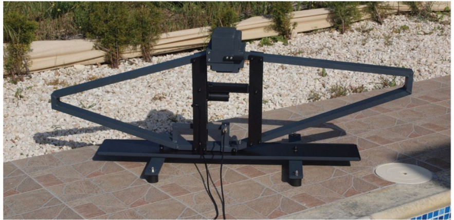
The Ciro-Mazzoni Stealth Antenna , chosen for portable operating on the Akamas peninsula.
