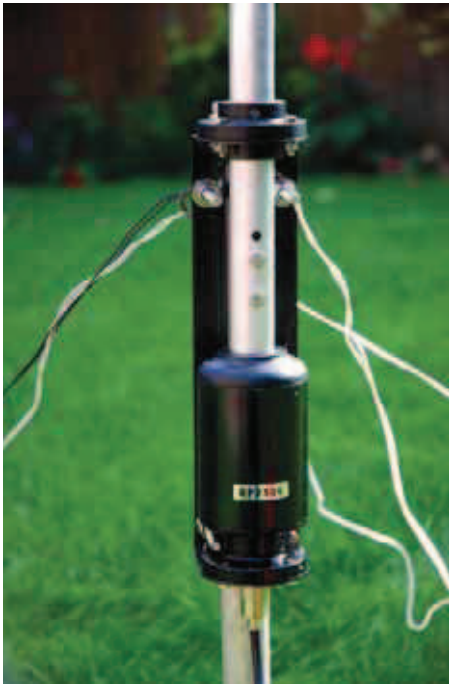
PHOTO 2: At the bottom of the antenna is a sealed matching unit with an SO239 socket for connection to the coax.
