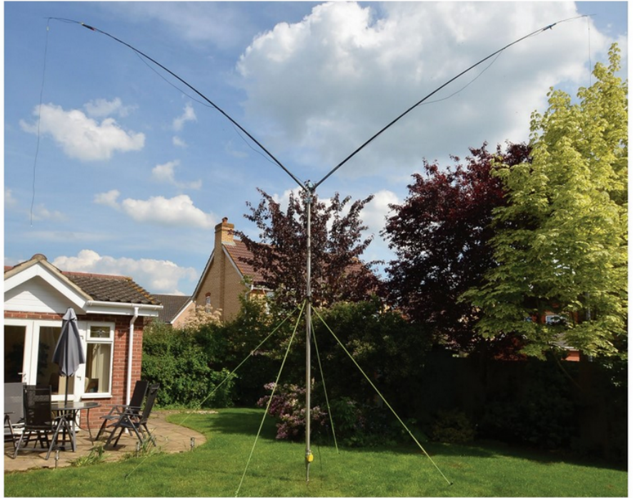
The DMV-II 80m antenna gets you onto 3.5MHz with a 'wingspan' of only about eight metres.
