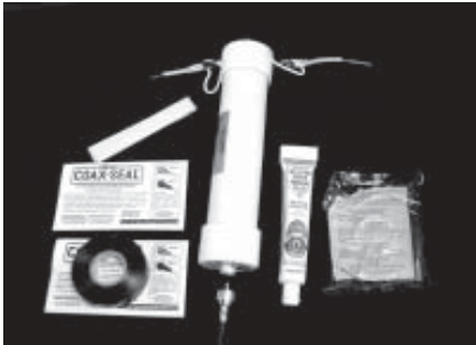
You need Coax Seal, STUF, Cold-shrink and electrical tape
