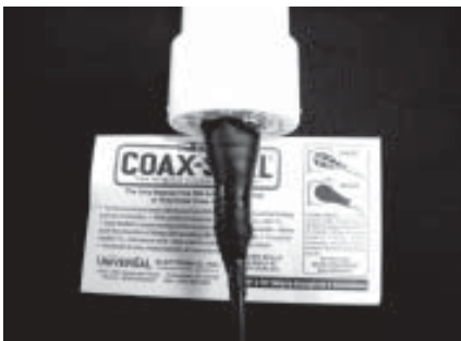
Apply one overlapping layer of Coax Seal. Press so that it sticks to the device and covers at least 1" of cable. The seal must be solid from device to cable.
