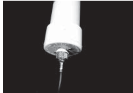
When connector is tightened, "STUF" is compressed and forced to fill any voids in the connectors. Moisture and excess STUF is forced out.
