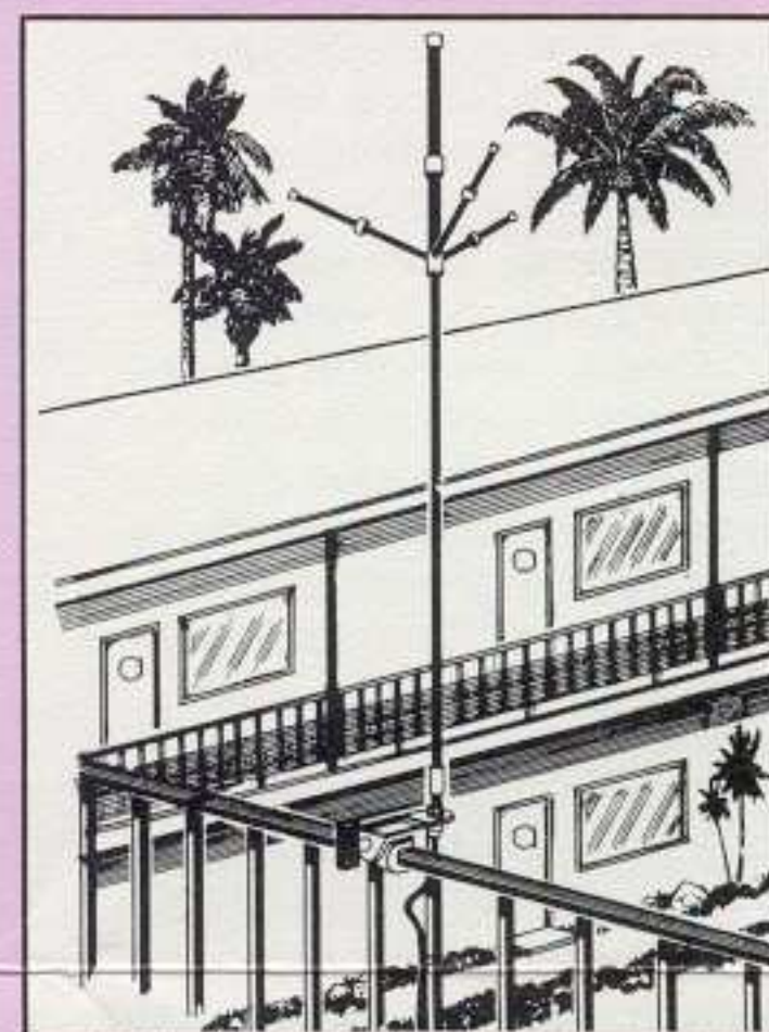
One possible installation to fit an unusual application: on balcony using railing for ground.
