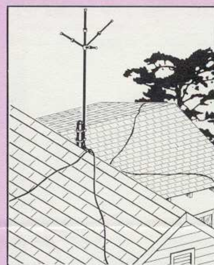
Roof mounted installation with ground radial system.
