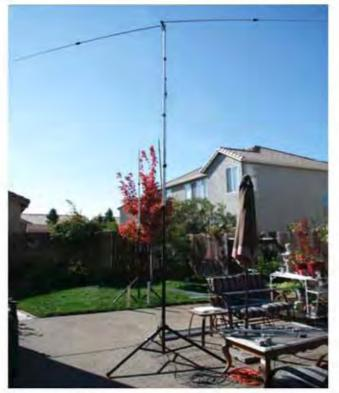
6 Band Rotatable Dipole 20, 15, 17, 12, 10, 6M **FALCON**.
