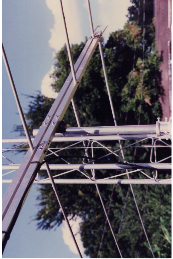
These photos show proper element phase reversal and attachment of the coax to the lower boom.
