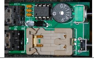
If you built your kit with the battery holder (recommended), locate the battery and remove it from its protective packaging. Note that the flat side is marked with a plus sign (+). This side will be up when the battery is inserted into the battery holder. Insert the battery into the battery holder. If you have done everything right, you should hear the keyer send "73" in Morse code through the speaker. Congratulations! Your kit is complete.
