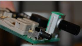
Install the two stereo jacks in the locations indicated on the component side of the PCB. Be sure to press them far enough in to get them fully seated. There are three plastic "bumps" on the bottom that will fit into holes in the PCB when they are pushed all the way in. Install the two threaded, knurled collars on the two stereo jacks. This keeps them from getting lost! You can use them to mount your PicoKeyer in a box or tin.
