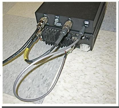
Connect the antenna feedline coax to the "ANT" jack on the rear of the IT-100.
