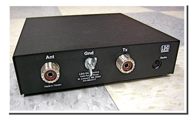
**ANT connector:** Connect the 50-ohm coax antenna feedline to this standard SO-239 connector.
