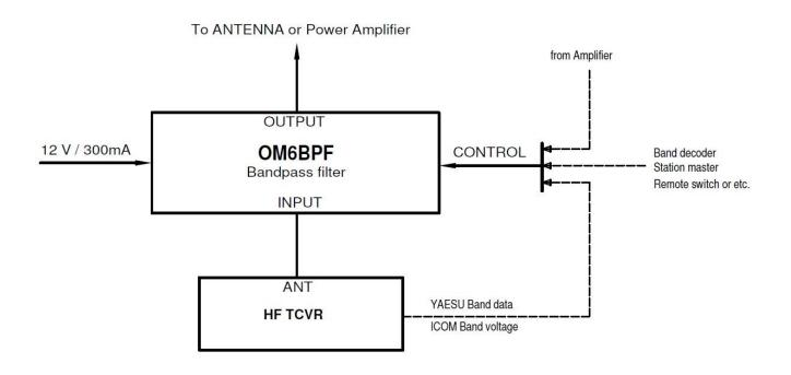
OM6BPF's INPUT socket connects to your TRX using a coax cable of 50 Ohms impedance where OUTPUT sockets shall be connected to either amplifiers input or directly to an matched antenna. OM6BPF has power rating of 200W so it should be always connected between TRX and PA!
