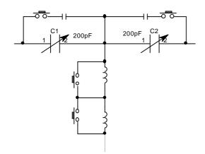
C1, C2 = 200 pF max, 3 kV L = Switched by relays Fixed C = Mica caps., 3 kV
