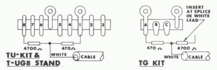
Insert 4700 ohms in series with the WHITE cable lead. Shunt 470 ohms from WHITE cable lead to ground.
