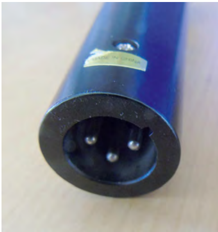
Fig. 5: XLR3 connector on the back of the M629 microphone.
