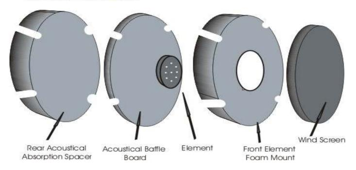
Instructions to install the MC-320 replacement element kit for an Astatic D104 head. **Note:** The microphone element now has pre-soldered wires to the element and each element has been test for audio response.
