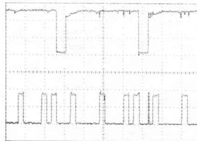
CS1 U4-20 (Synchronizing Signal) V = 2.0 V/div H = 2 uS/div Baseline at division 5 A13 U1-3 V = 2.0 V/div H = 2 uS/div Baseline at division 1
