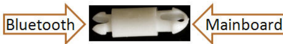
Figure 5: Bluetooth module fastening standoff
