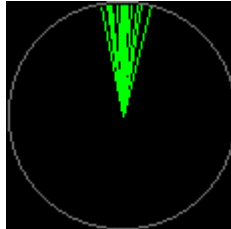
BPSK Signal too high in frequency.
