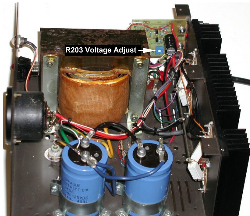
Figure 6. View of Figure 5 from the other side. Note in this case R203 is a top adjust, allowing voltage adjustment to be made from the inside of the power supply. A side adjust pot can be used so the adjustment may be made from the top, however, the adjustment will be backward i.e., CW decreases output voltage and CCW increases output voltage.
