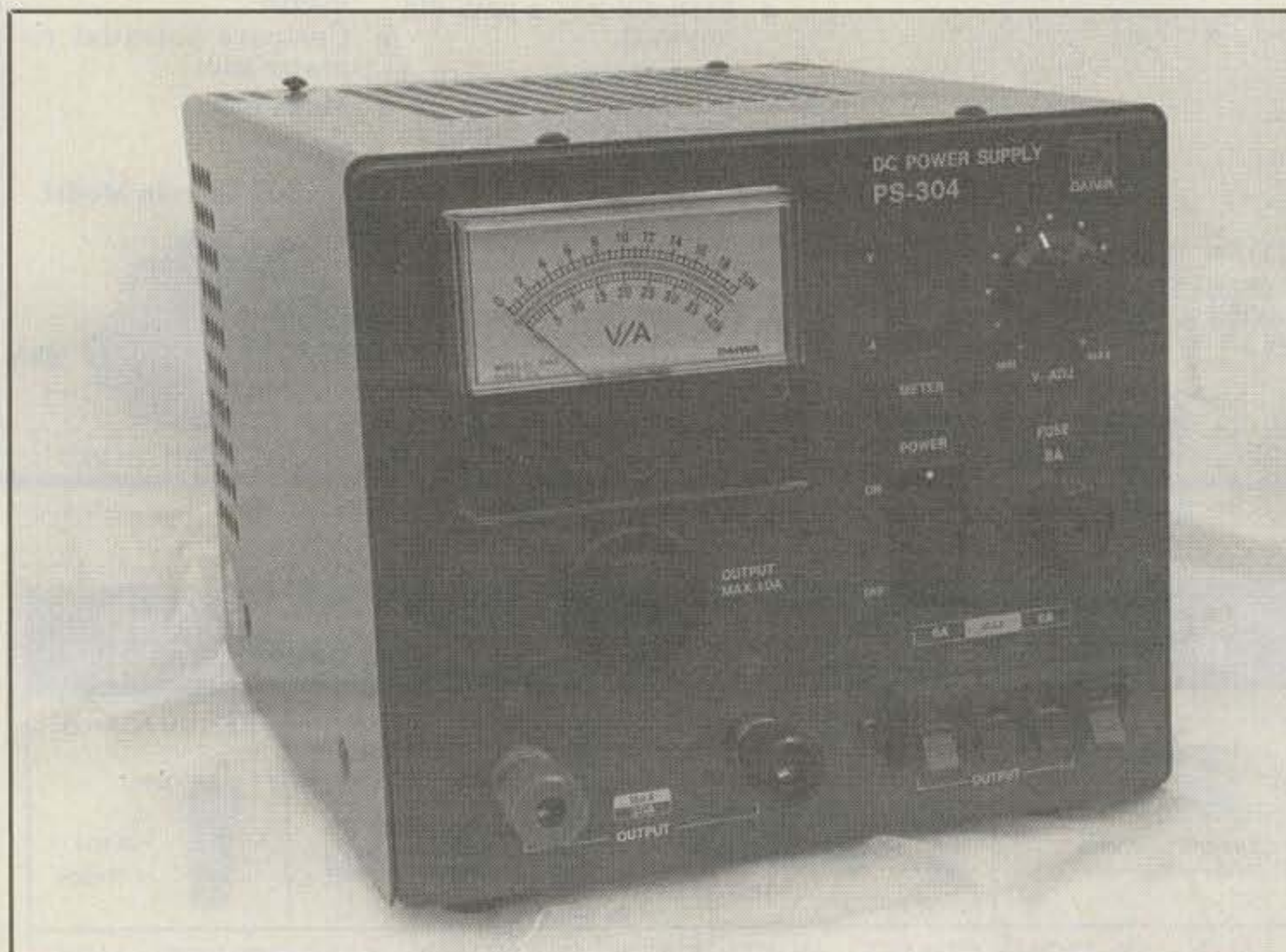
Front view of the Daiwa PS-304 power supply. At the upper left is the meter and immediately below is the cigarette-plug receptacle. The high-output terminals are at the lower right.
