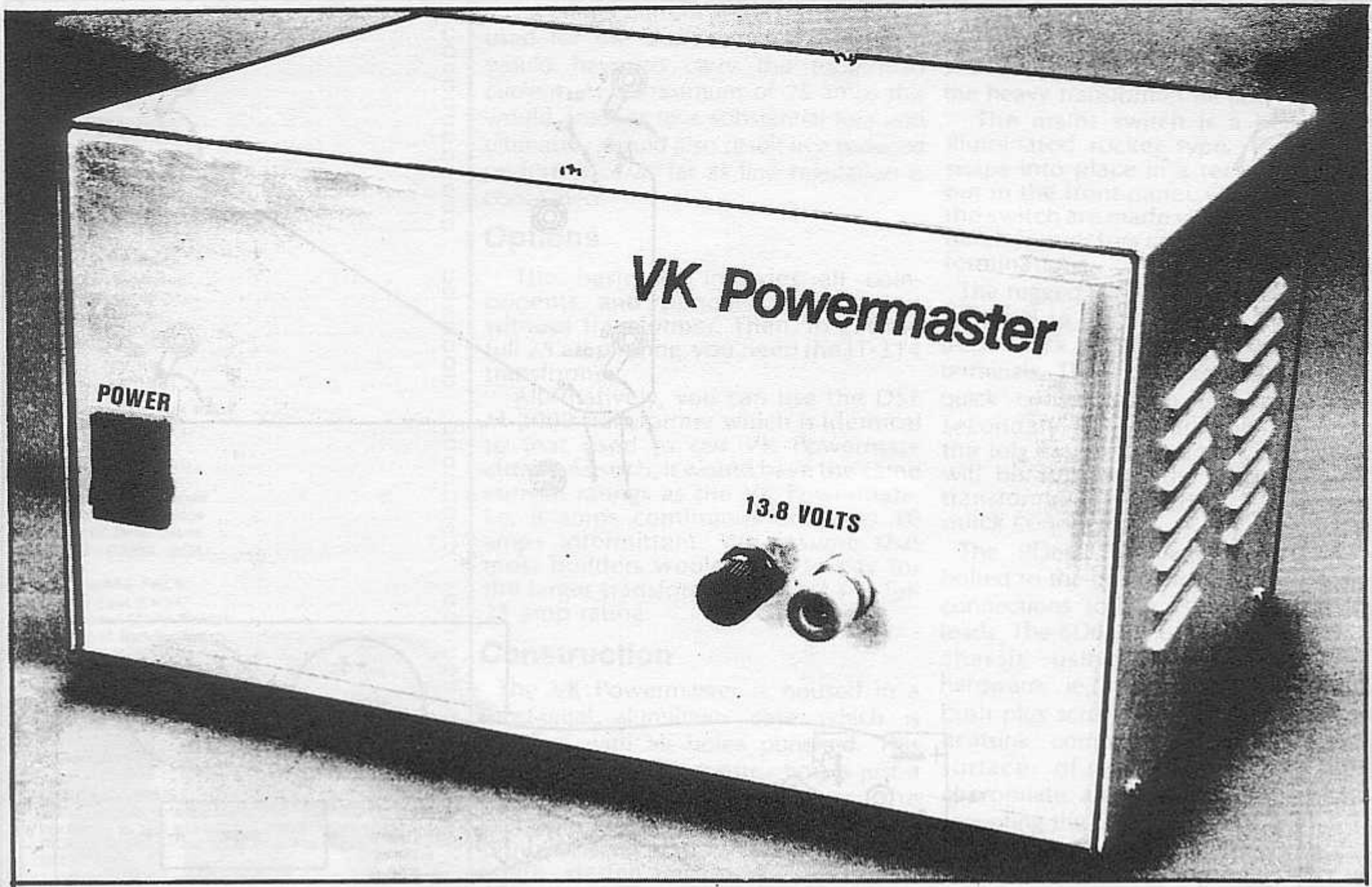
The above photograph shows the assembled kit. The louvred top cover aids heat dissipation.
