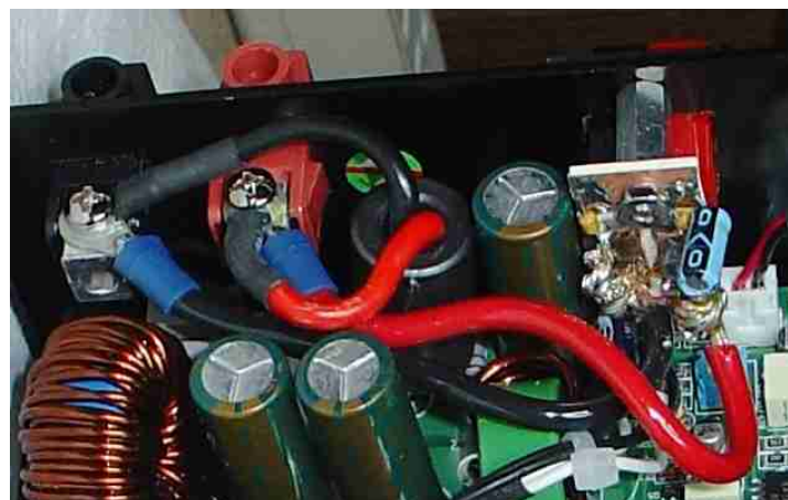
Photo J: Connector assembly mounted in place.
