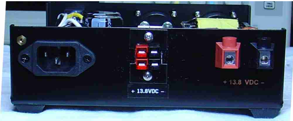
Photo K: SEC-1235M back panel with Powerpole™ connectors mounted
