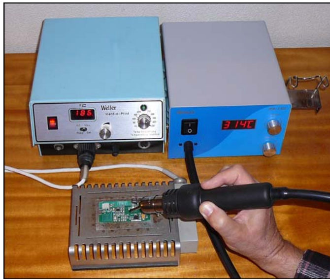
Fig. 10 Hot air soldering
