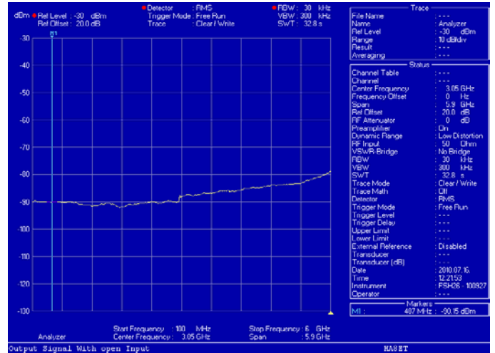
Fig. 22 Output signal with open input (between 100 MHz and 6 GHz), box covered
