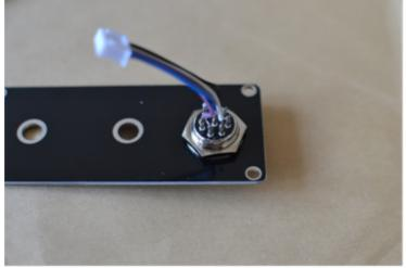
[ ] Make sure both controls have a nut on first. Plug in the microphone cable into the SIP5 socket on board, install the front panel using two black chassis screws, protrude the LED and two controls from front panel holes, then put a washer and another nut on each control, and finally install the knobs.
