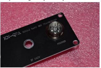
[ ] Solder the microphone cable, based on the schematic below. This connection is compatible with ICOM HM-series and the supplied optional microphone. To use a different brand microphone, please identify the pinout and wire it accordingly. On the SIP5 connector pin 1 is SPEAKER, pin 2 is GND, pin 3 is MIC, pin 4 is PTT, and pin 5 is +8VT.
