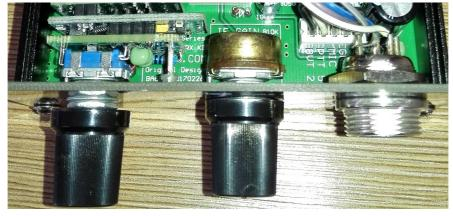
[ ] Preset the IF GAIN control to mid-way and you are ready to start alignment. After alignment, remember to install the top chassis using another 4x black chassis screws.
