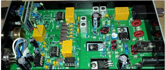
Prepare the front panel by installing the 8-pin microphone connector.
